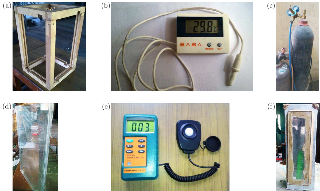
Fig. 5. Experimental accessories (a) glass supporting structure, (b) digital thermometer, (c) argon cylinder, (d) separator, (e) solar power meter and (f) argon-oxygen separator
