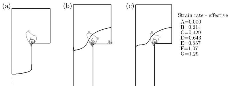
Fig. 3. Strain rates describing the beginning of weld creation during axisymmetrical forward extrusion through a rectangular die: (a) extrusion of a single billet, (b) welding with  $m = 0.4$  at the billets interface, (c) welding with  $m = 0.9$
