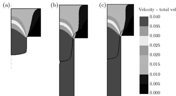
Fig. 17. Velocity distributions during forward extrusion through a rectangular die with a spherical face of the upper billet: (a) extrusion of a single billet, (b) welding with  $m = 0.4$  at the billets interface, (c) welding with  $m = 0.9$
