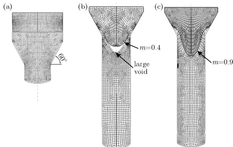
Fig. 8. Joining during forward extrusion through a conical die: (a) view of billets before joining, (b) welding with  $m = 0.4$  at the billets interface, (c) welding with  $m = 0.9$
