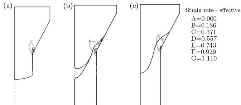
Fig. 9. Strain rates for the beginning of weld creation while forward extrusion through a conical die: (a) extrusion of a single billet, (b) welding with  $m = 0.4$  at the billets interface, (c) welding with  $m = 0.9$
