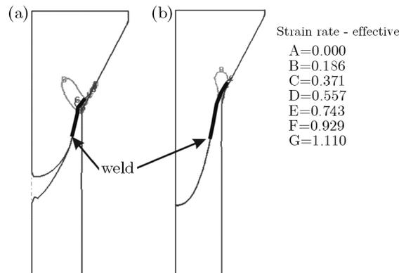
Fig. 10. Strain rates for the end of weld creation while forward extrusion through a conical die: (a) welding with  $m = 0.4$  at the billets interface, (b) welding with  $m = 0.9$
