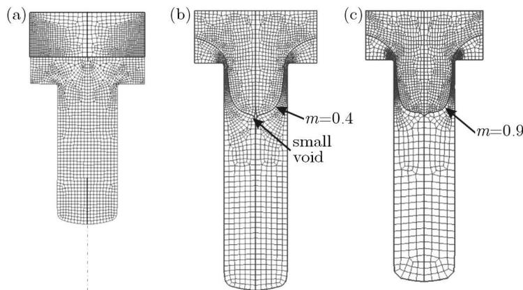
Fig. 2. Joining during forward extruding through a rectangular die: (a) view of billets before joining, (b) welding with  $m = 0.4$  at the billets interface, (c) welding with  $m = 0.9$  at the billets interface
