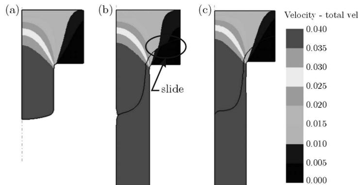
Fig. 7. Velocity distributions while forward extrusion through a rectangular die: (a) extrusion of a single billet, (b) welding with  $m = 0.4$  at the billets interface, (c) welding with  $m = 0.9$
