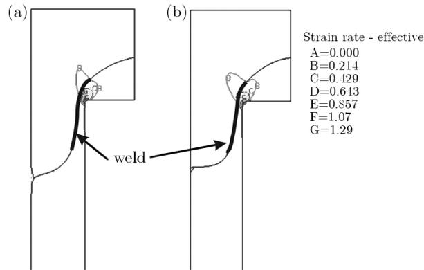
Fig. 4. Strain rates describing the end of weld creation during axisymmetrical forward extrusion through a rectangular die: (a) welding with  $m = 0.4$  at the billets interface, (b) welding with  $m = 0.9$
