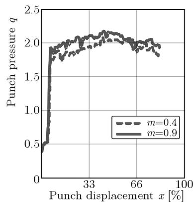
Fig. 5. Punch pressures obtained during forward extrusion through a rectangular die
