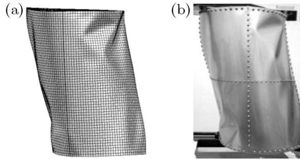
Fig. 8. The advanced post-critical deformation of the examined structure (a) and the distribution of contour lines representing size of the deformation found by making use of the Moiré projection method (b)
