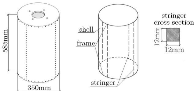
Fig. 7. A schematic view of a complete cylindrical shell reinforced by four members and a schematic view of the structure including dimensions
