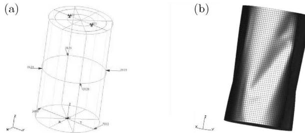
Fig. 9. A geometrical model of a structure made in MSC PATRAN environment with boundary conditions and loading (a). The incorrect form of deformation obtained in the case of too many elements (b)
