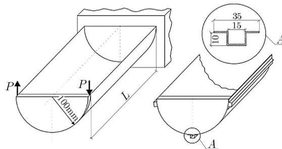
Fig. 2. A schematic view of the tested structure
