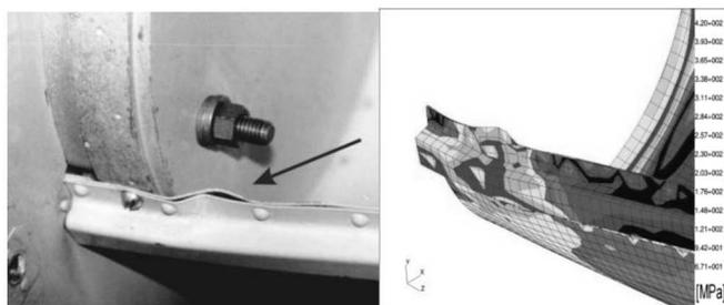
Fig. 3. A comparison of the deformation forms obtained experimentally and numerically
