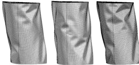
Fig. 5. Incorrect forms of shell stability loss, showing member buckling not revealed in the experiment
