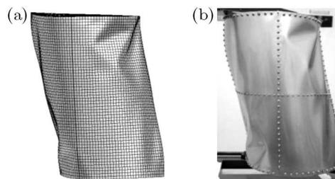
Fig. 6. Accepted as a satisfactory form of post-critical deformation obtained from nonlinear analysis (a) and a deformation form obtained from experimental tests at the identical load (b)
