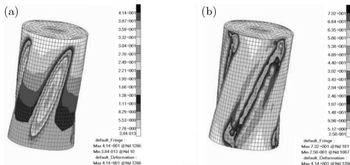
Fig. 10. The deformation distribution (a) and reduced stress distribution according to Huber-Mises hypothesis (b) for 100% of the maximum load (stringers modelled with thick shell elements)
