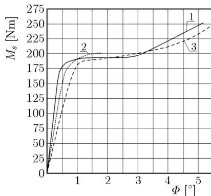
Fig. 11. The presentation of the representative equilibrium paths; 1 – experiment, 2 – numerical analysis – stringers modelled with beam elements, 3 – numerical analysis – stringers modelled with shell elements
