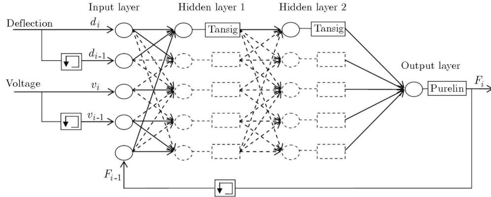
Fig. 1. Structure of the proposed neural network model
