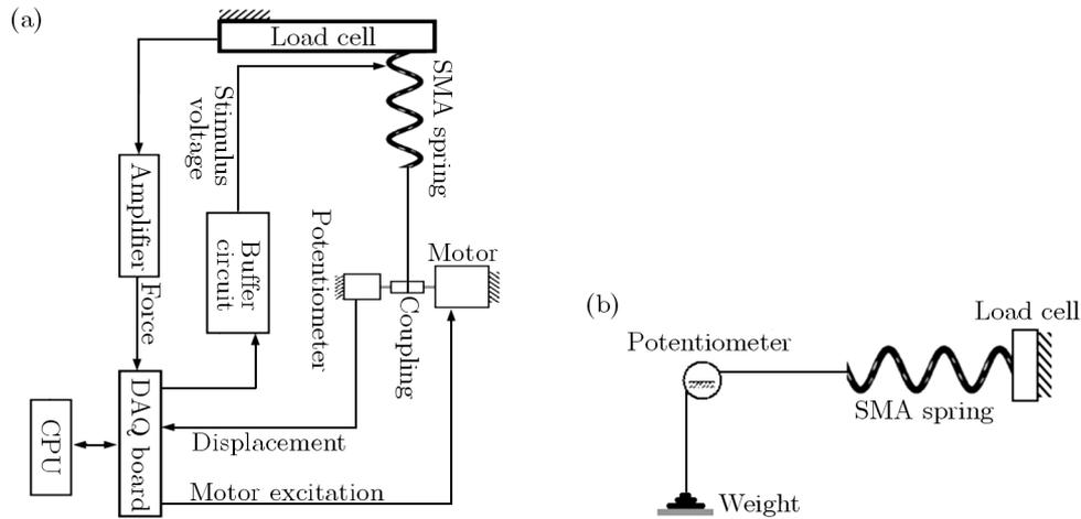
Fig. 3. Schematic overview of the setup; (a) top view with electronic circuit (fixed-voltage and fixed-length tests), (b) side view (fixed-stress tests)
