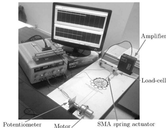
Fig. 2. SMA spring test bed
