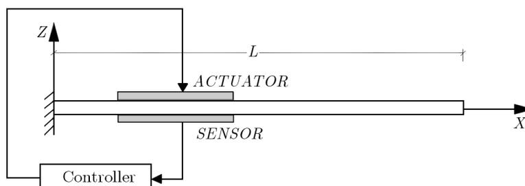
Fig. 1. Configuration of the beam with piezoelectric patches
