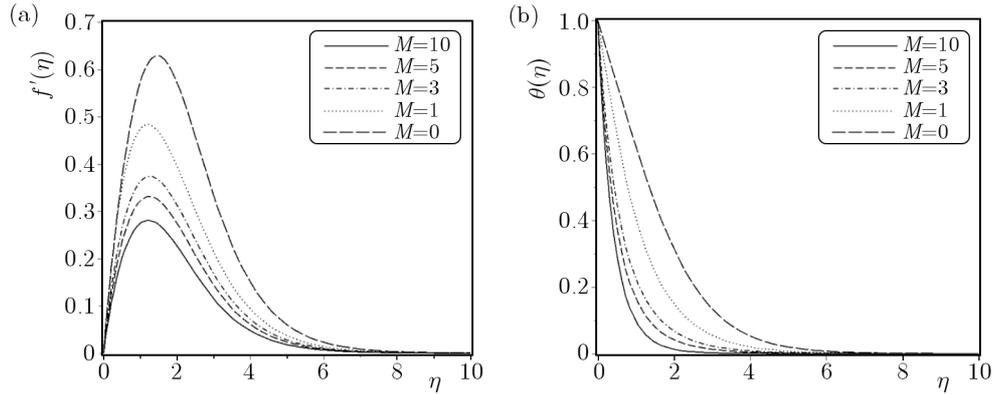
Fig. 2. Velocity profiles  $f'(\eta)$  (a) and temperature profiles  $\theta(\eta)$  (b) for  $Pr = 1$  and different values of  $M$
