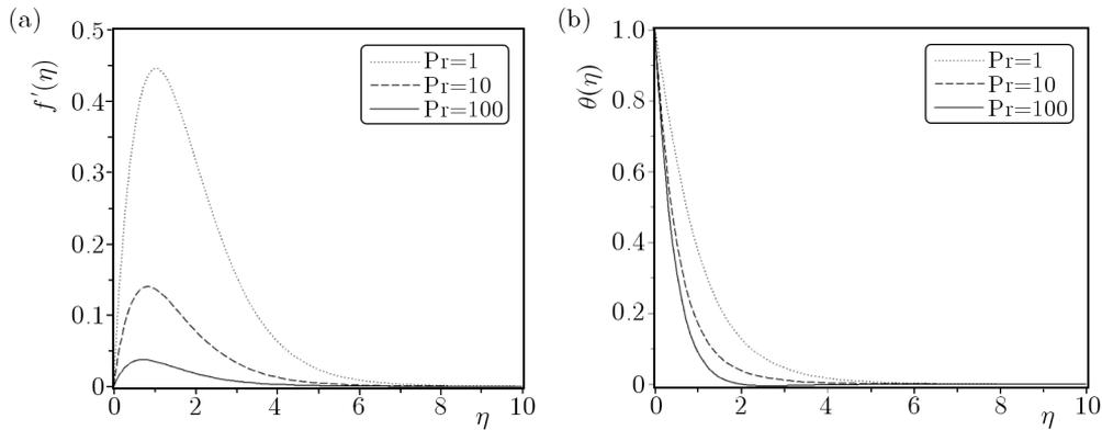
Fig. 3. Velocity profiles  $f'(\eta)$  (a) and temperature profiles  $\theta(\eta)$  (b) for  $M = 2$  and different Prandtl numbers
