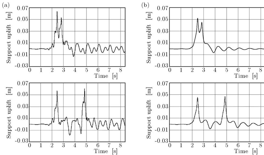
Fig. 11. Typical steady-arm uplift in catenaries with different proportional damping for two different separations of pantographs: (a)  $\alpha = 0.00275$ ; (b)  $\alpha = 0.0275$
