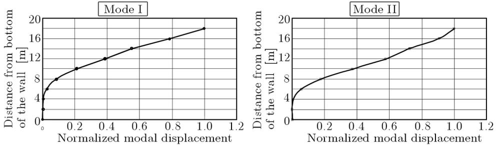
Fig. 1. Mode shapes of the wall at its fundamental frequencies
