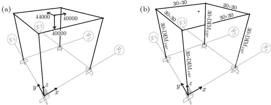
Fig. 2. FE model for the performance assessment of SOBI in the case of closely spaced modes: mass assignment (a), sections (b)
