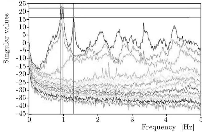
Fig. 5. The School of Engineering Main Building (Naples): RC0 record – Singular Value plot
