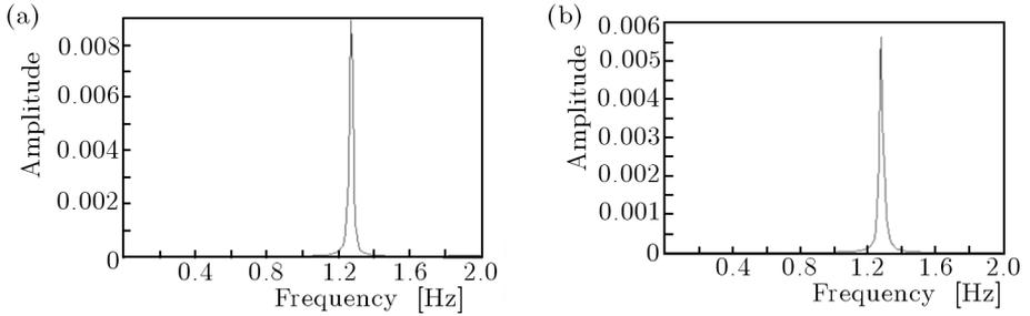
Fig. 4. Nearly repeated frequencies: spectra of the sources at 1.27 Hz (a) and 1.28 Hz (b)
