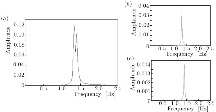
Fig. 3. 17% modal overlap: cross-spectrum between two orthogonal measurement directions (a) and extracted sources corresponding to the first (b) and second (c) mode
