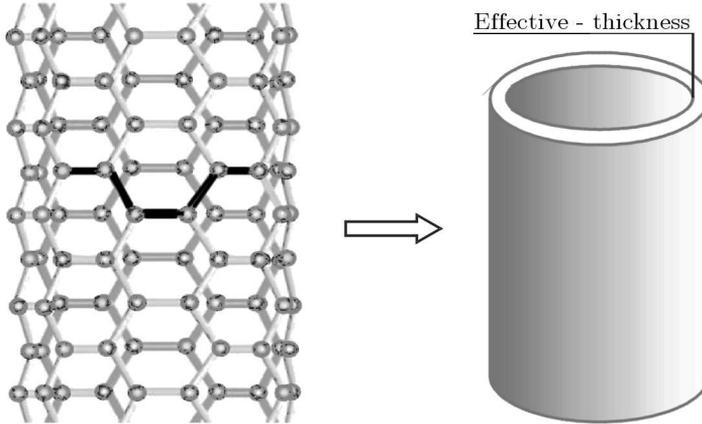
Fig. 2. Continuum model of carbon nanotube structure
