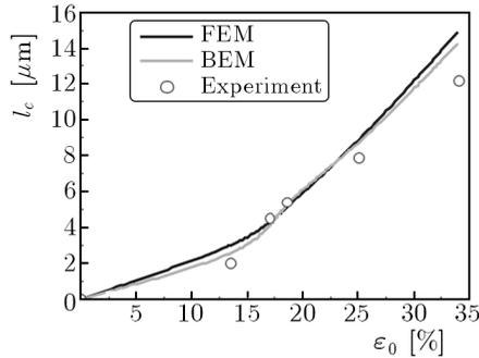
Fig. 4. Measured average interface debond length  $l_e$  as a function of the applied strain  $\varepsilon_0$  versus calculated interface debond length for the zinc coating shear strength  $\tau^{cr} = 180$  MPa
