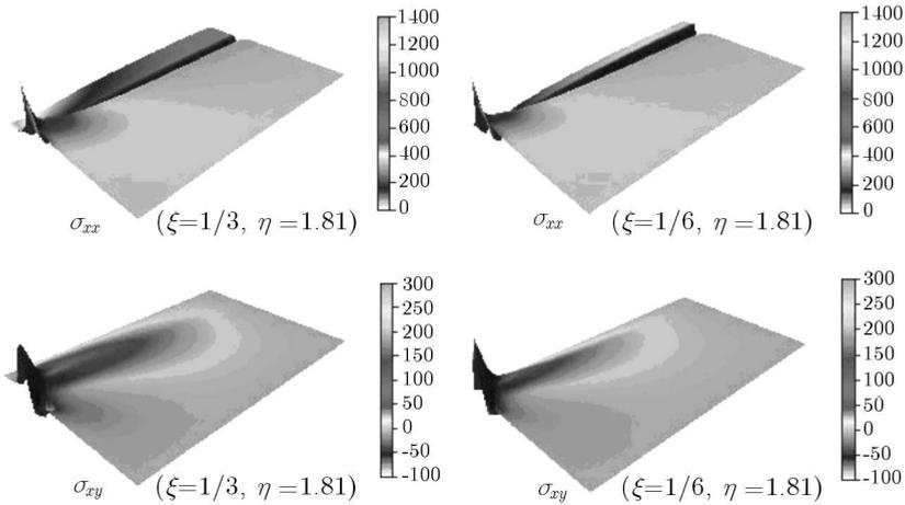
Fig. 3. Plots of stresses  $\sigma_{xx}(x, y)$ ,  $\sigma_{xy}(x, y)$  for the pre-cracked bimaterial structure for different thickness ratios  $\xi = h_A/h_B$  and the elastic moduli ratio  $\eta = 1.81$
