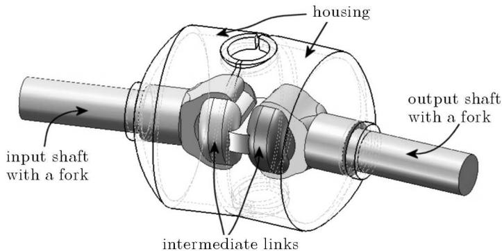
Fig. 1. Tracta joint assembly
