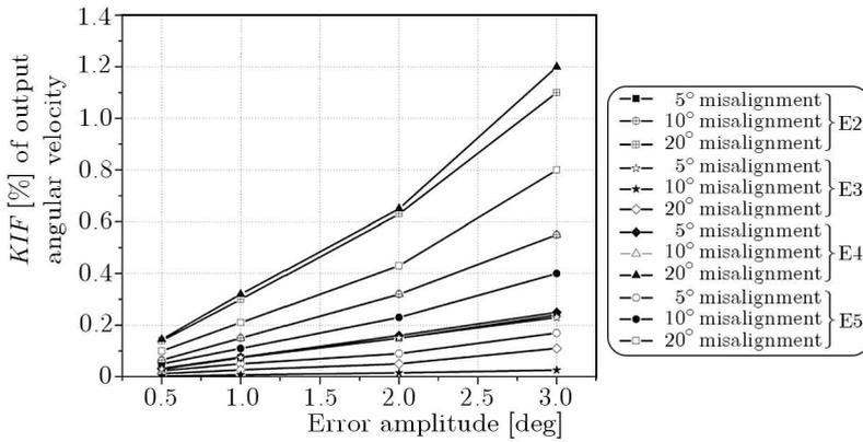
Fig. 15. Design chart of the angular errors  $KIF$ s of the output shaft angular velocity
