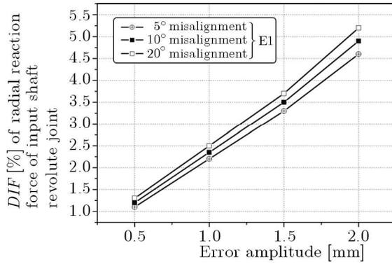
Fig. 19. Design chart of the linear errors *DIFs* on the radial reaction force of the input shaft revolute joint
