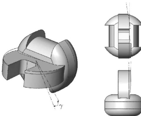
Fig. 8. General angular error combines the effects of the two degrees of freedom
