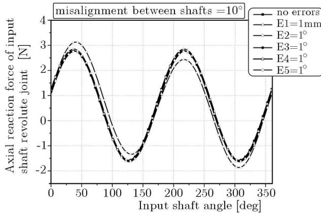
Fig. 13. Irregularities of the axial force of the input shaft revolute joint due to errors for the misalignment between shafts 10°
