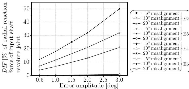
Fig. 17. Design chart of the angular errors  $DIF$ s of the radial reaction force of the input shaft revolute joint
