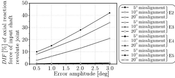
Fig. 18. Design chart of the angular errors *DIFs* on the axial reaction force of the input shaft revolute joint
