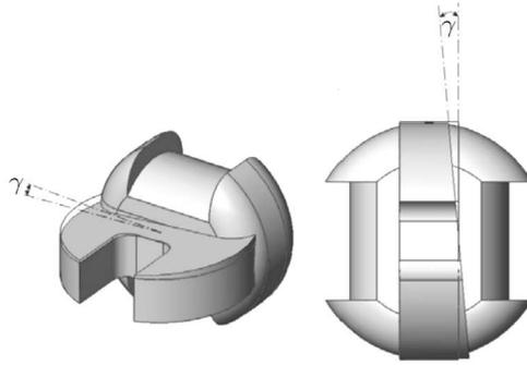
Fig. 6. First degree of freedom of the slot surface due to planarity or an angular error
