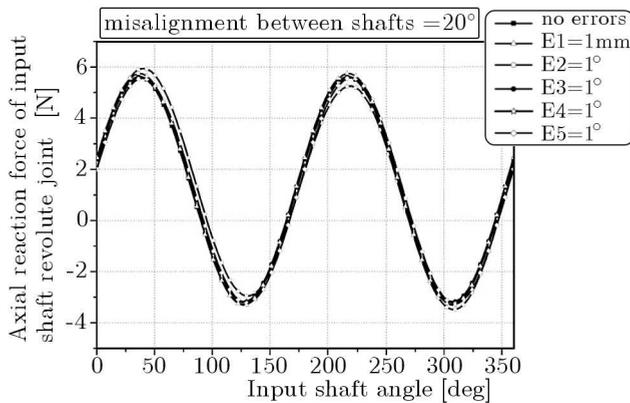
Fig. 14. Irregularities of the axial force of the input shaft revolute joint due to errors for the misalignment between shafts 20°
