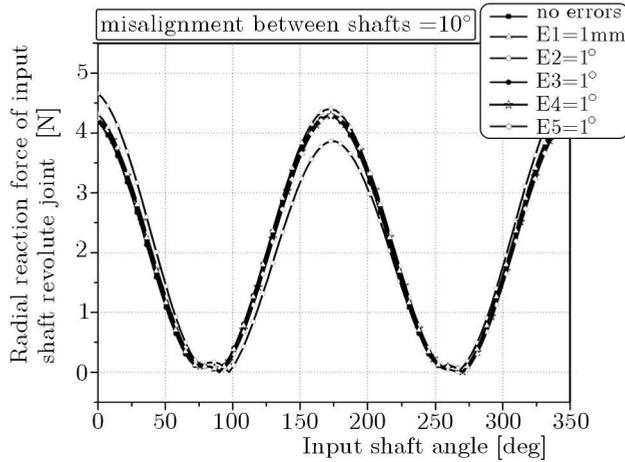
Fig. 11. Irregularities of the radial force of the input shaft revolute joint due to errors for the misalignment between shafts  $10^\circ$
