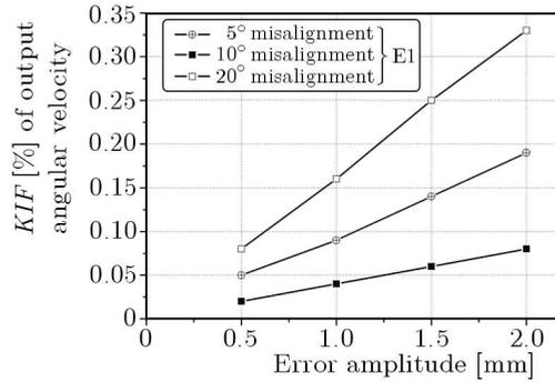
Fig. 16. Design chart of the linear error  $KIF$ s of output shaft angular velocity
