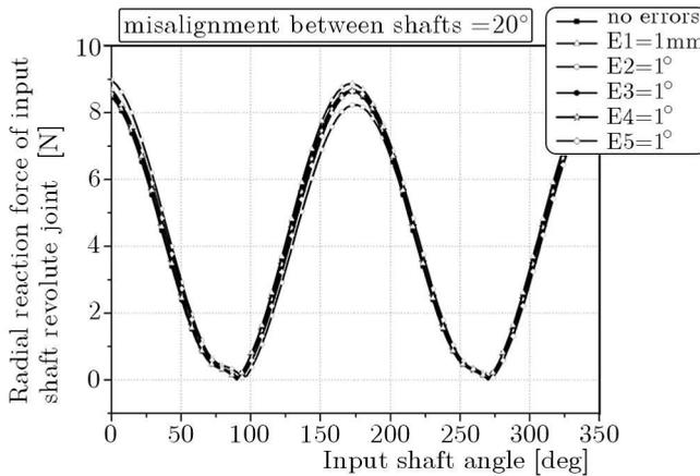
Fig. 12. Irregularities of the radial force of the input shaft revolute joint due to errors for the misalignment between shafts  $20^\circ$
