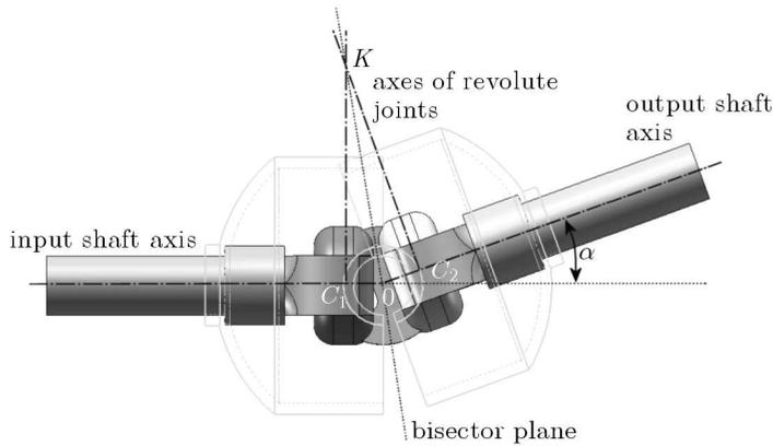
Fig. 3. Geometrical condition for a homokinetic Tracta joint
