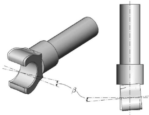
Fig. 5. Angular error of the fork axis
