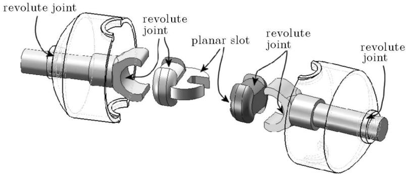
Fig. 2. Tracta joint exploded view
