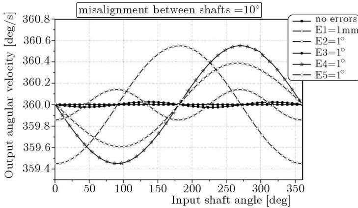
Fig. 9. Kinematic irregularities due to errors when the misalignment between the two shafts is  $10^\circ$
