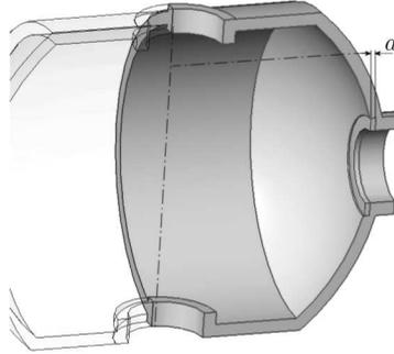
Fig. 4. Position error of the lateral surface of the bearing housing
