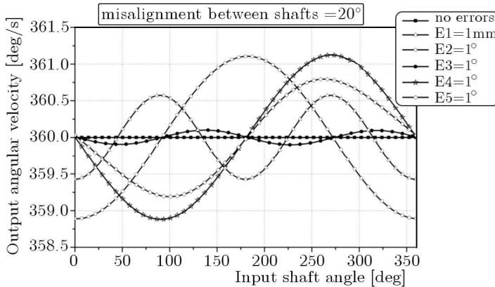
Fig. 10. Kinematic irregularities due to errors when the misalignment between the two shafts is  $20^\circ$
