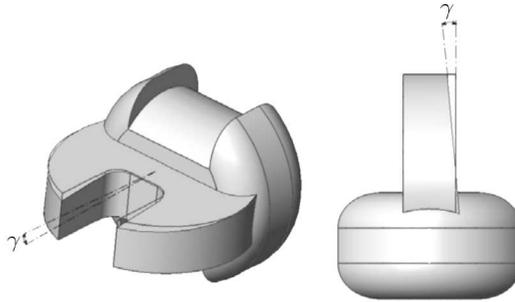
Fig. 7. Second degree of freedom of the slot surface due to planarity or an angular error
