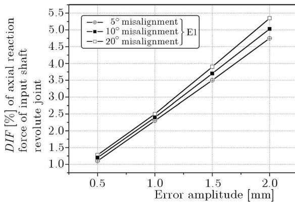
Fig. 20. Design chart of the linear errors *DIFs* of the axial reaction force of the input shaft revolute joint
