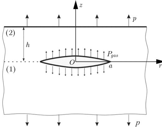
Fig. 1. A half-space with a gas-filled penny-shaped crack
