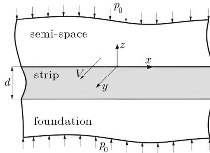
Fig. 1. Scheme of the contact system
