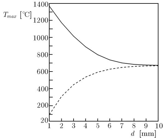
Fig. 8. Dependence of the maximum temperature  $T_{max}$  on the strip thickness  $d$
