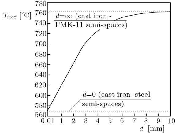
Fig. 4. Dependence of the maximum contact temperature  $T_{max} = T(0, t_{max})$  on the strip thickness  $d$
