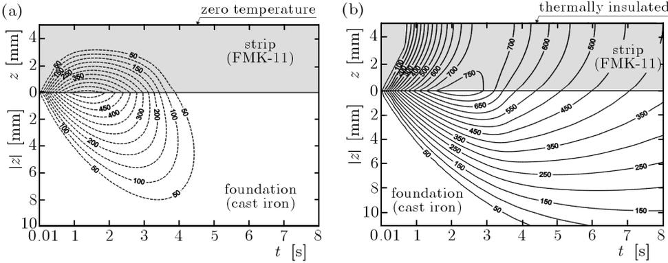
Fig. 6. Isolines of the temperature  $T$  [ $^{\circ}\text{C}$ ] at  $t_s = 3.44$ s
