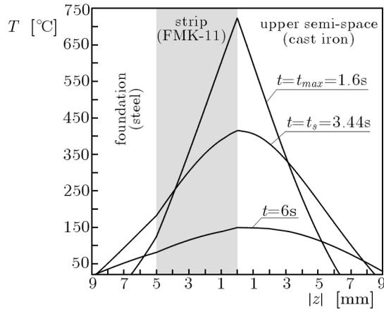
Fig. 3. Temperature distribution along the distance  $|z|$  from the contact surface at three time moments
