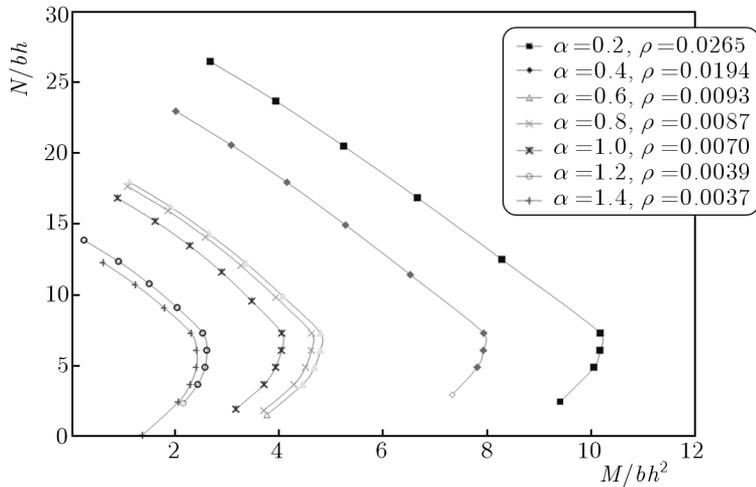
Fig. 5. Interaction curves at  $d/h = 0.95$  and  $\beta = 4.5$
