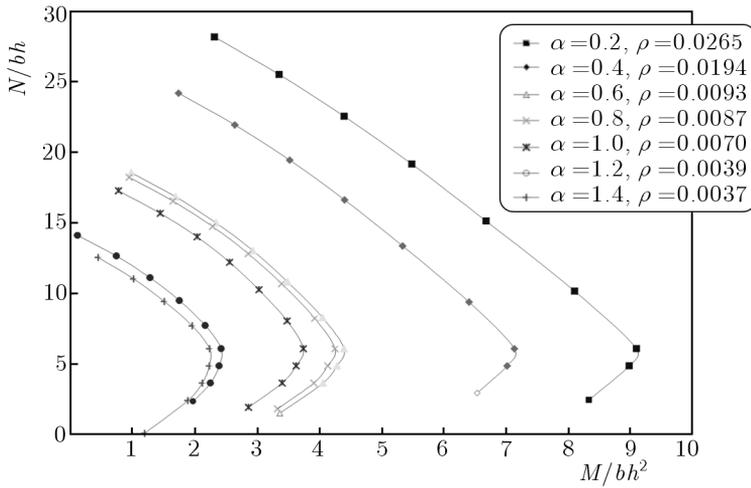
Fig. 3. Interaction curves at  $d/h = 0.85$  and  $\beta = 4.5$
