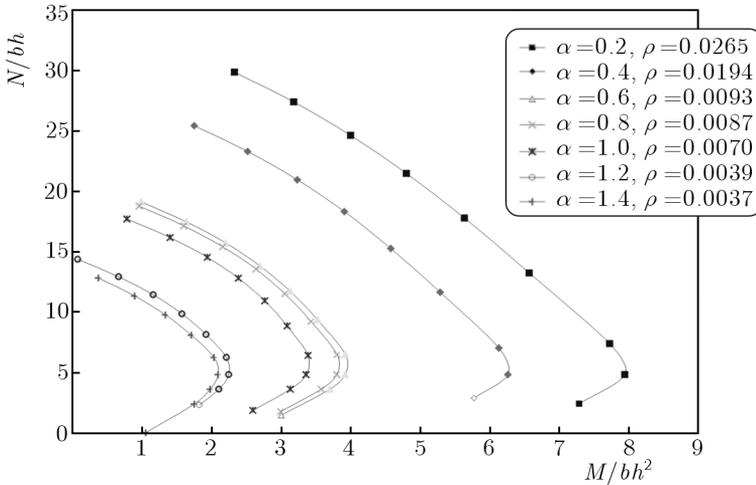
Fig. 1. Interaction curves at  $d/h = 0.75$  and  $\beta = 4.5$
