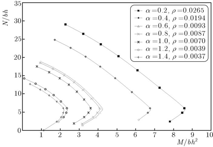
Fig. 2. Interaction curves at  $d/h = 0.8$  and  $\beta = 4.5$
