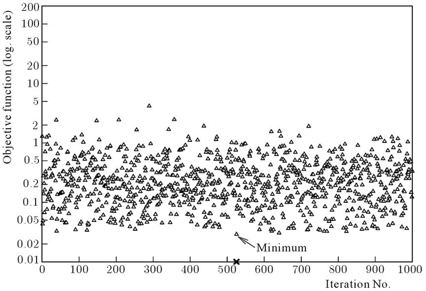
Fig. 3. Objective function vs. iteration number – tabu search, 3-parameter empirical equation for water transport in corn kernels, relative humidity 50%
