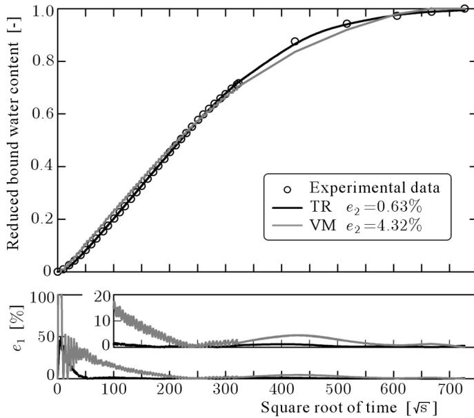
Fig. 7. Similarity between experimental data and results predicted by the operational finite element model with four coefficients estimated by the variable metric (VM) and trust region (TR) algorithms. The relative errors are denoted by  $e_2$  (global) and  $e_1$  (local). The model corresponds to the transient bound water diffusion in Scots pine wood
