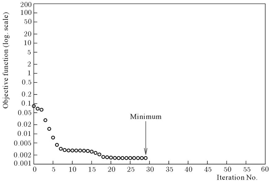
Fig. 6. Objective function vs. iteration number – estimation of four coefficients by the trust region algorithm, the operational finite element model corresponds to the transient bound water diffusion in Scots pine wood
