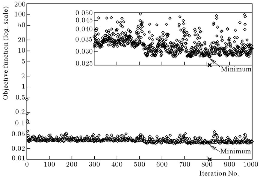
Fig. 4. Objective function vs. iteration number – genetic algorithm, 3-parameter empirical equation for water transport in corn kernels, relative humidity 50%
