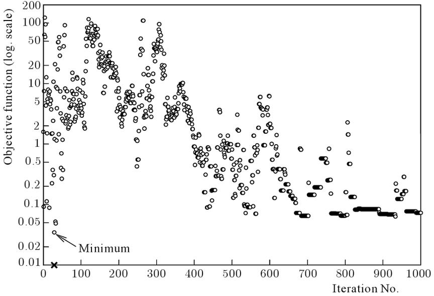
Fig. 2. Objective function vs. iteration number – simulated annealing, 3-parameter empirical equation for water transport in corn kernels, relative humidity 50%
