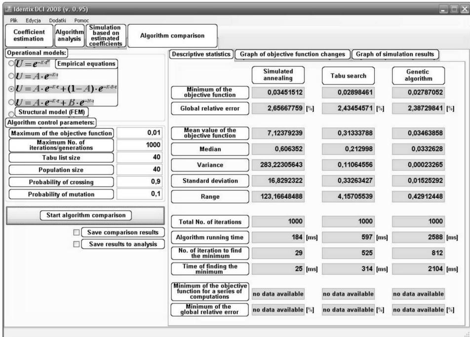
Fig. 1. An interface of the software module for assessing performance of optimization algorithms
