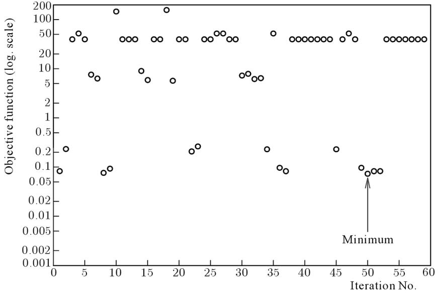
Fig. 5. Objective function vs. iteration number – estimation of four coefficients by the variable metric algorithm, the operational finite element model corresponds to the transient bound water diffusion in Scots pine wood
