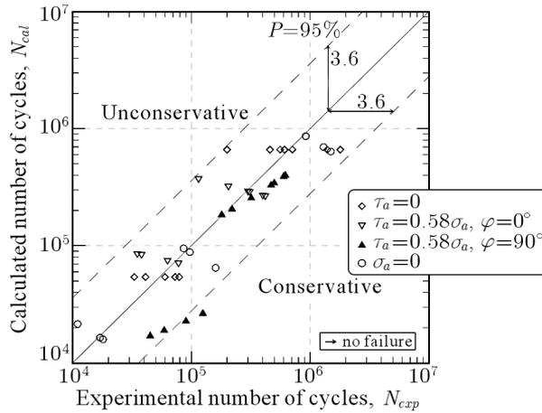
Fig. 8. Comparison of fatigue life  $N_{cal}$  calculated according to Eq. (2.17) and experimental fatigue life  $N_{exp}$  for Fe-Cu-Ni<sup>(3)</sup> sintered steel
