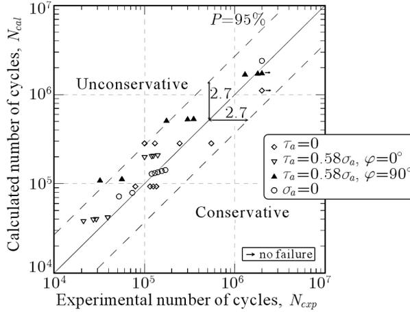
Fig. 6. Comparison of fatigue life  $N_{cal}$  calculated according to Eq. (2.17) and experimental fatigue life  $N_{exp}$  for Fe-Cu-Ni<sup>(1)</sup> sintered steel
