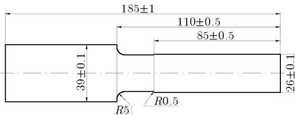
Fig. 3. Geometry of the round specimen
