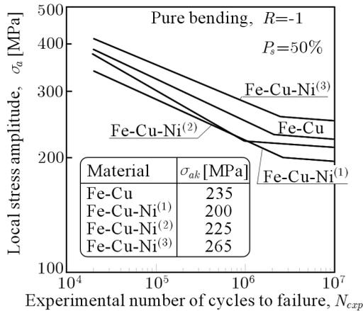
Fig. 4. S-N curves for alternating bending
