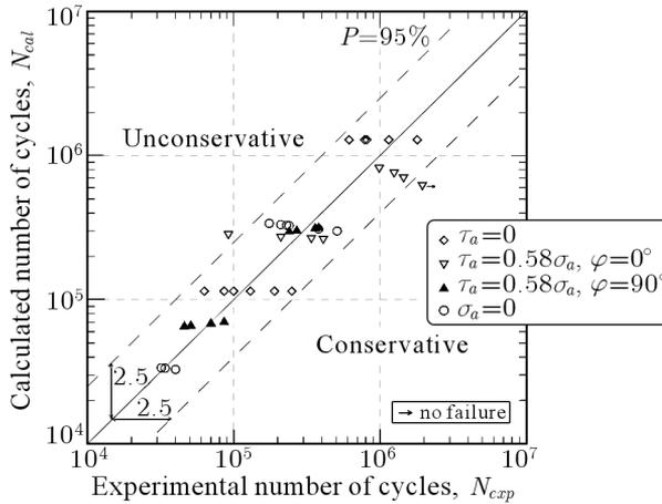
Fig. 7. Comparison of fatigue life  $N_{cal}$  calculated according to Eq. (2.17) and experimental fatigue life  $N_{exp}$  for Fe-Cu-Ni<sup>(2)</sup> sintered steel
