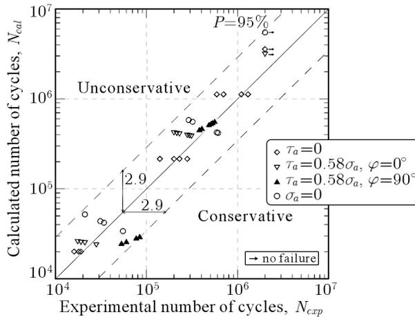
Fig. 5. Comparison of fatigue life  $N_{cal}$  calculated according to Eq. (2.17) and experimental fatigue life  $N_{exp}$  for Fe-Cu sintered steel
