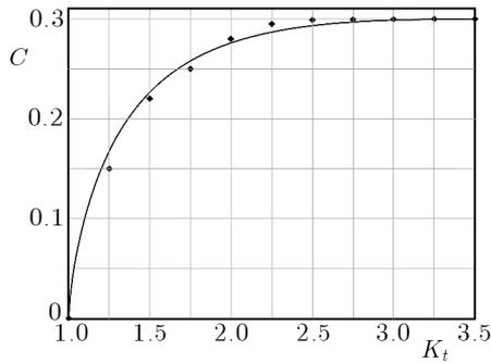
Fig. 1. Changes of coefficient  $C$  values against stress concentration factor  $K_t$
