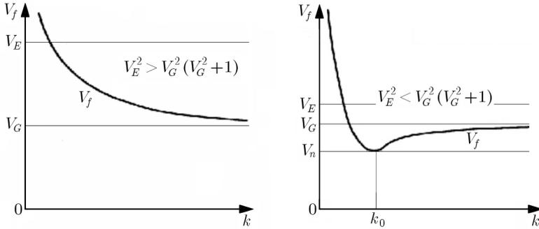
Fig. 5. Phase velocity  $V_f$  versus wave number  $k$  for two qualitatively different cases of the solution
