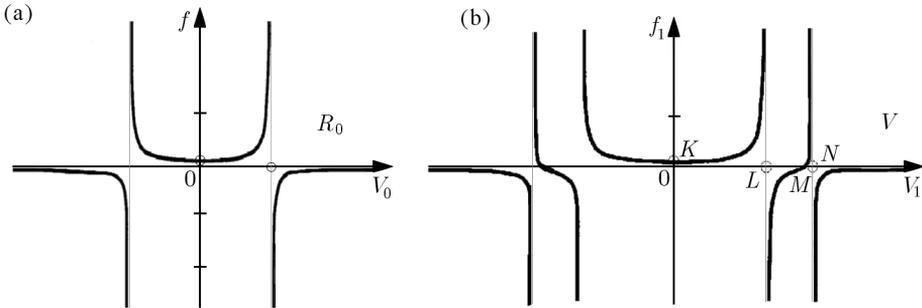
Fig. 7. (a) Function  $W_0/F_0 = f(V_0)$  for the Bernoulli-Euler beam, and (b) for the Timoshenko beam
