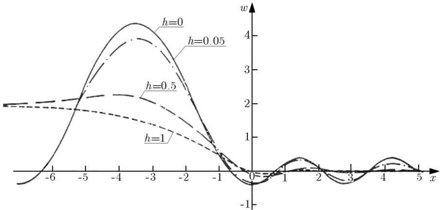
Fig. 4. Displacements of the Bernoulli-Euler beam on the Winkler foundation in the super-critical case ( $V = 1.2$ ) for various damping coefficients
