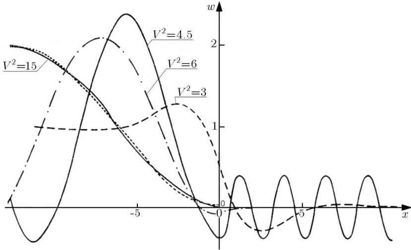
Fig. 6. Displacements of the Timoshenko beam on the Winkler foundation for various values of the load speed, in the case of parameters  $V_E^2 < V_G^2(V_G^2 + 1)$  (which was not considered by Achenbach and Sun, 1965)
