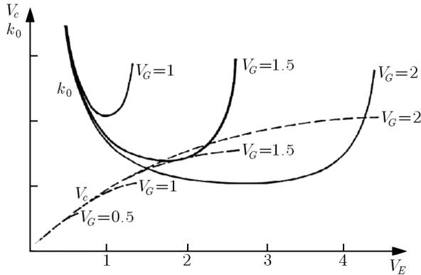
Fig. 8. Critical speed  $V_c$  and related wave number  $k_0$  versus the value of longitudinal wave  $V_E$  for selected values of  $V_G$
