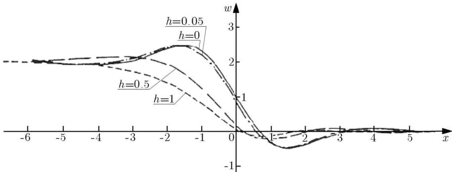
Fig. 2. Displacements of the Bernoulli-Euler beam on the Winkler foundation in the sub-critical case ( $V = 0.8$ ) for various damping coefficients
