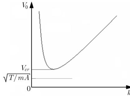
Fig. 1. Wave velocity  $V_0$  versus wave number  $k$  for the Bernoulli-Euler beam on the Winkler foundation subjected to longitudinal force  $T$
