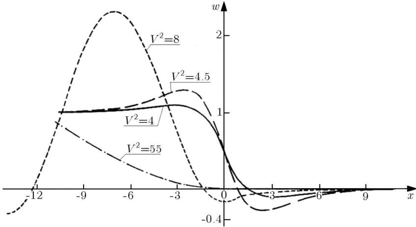
Fig. 3. Displacements of the Timoshenko beam on the Winkler foundation for various values of the load speed. The results are found for a parameter range similar to that used by Achenbach and Sun (1965)
