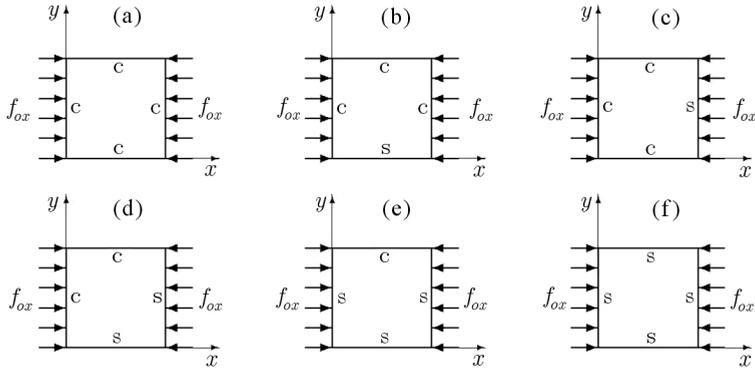
Fig. 1. Rectangular plate under uniaxial in-plane loading and boundary conditions
