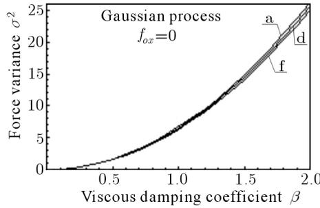
Fig. 2. Stability domains of a plate subjected to the uniaxial in-plane Gaussian parametric excitation for different boundary conditions,  $f_{ox} = 0$
