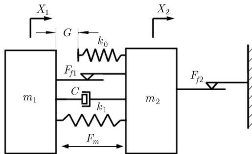
Fig. 2. Physical model of the electro-vibroimpact system (Ho *et al.*, 2008)
