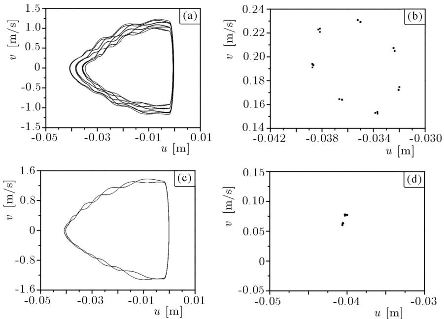
Fig. 4. Phase planes of relative motion of the bar at a control frequency of (a) 7 Hz and (c) 8 Hz. Poincaré maps are plotted for (b) 7 Hz and (d) 8 Hz
