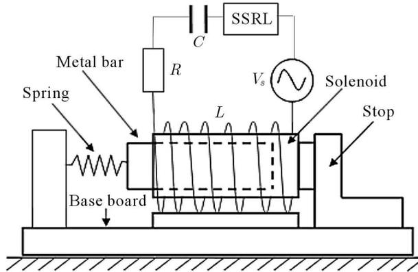
Fig. 1. Schematic diagram of the prototype of an electro-vibroimpact device (Nguyen, 2007)
