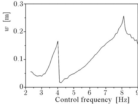
Fig. 5. The achieved mole progression for 5 seconds with respect to the control frequency obtained from numerical integration. The same set of parameters was used as in Fig. 3
