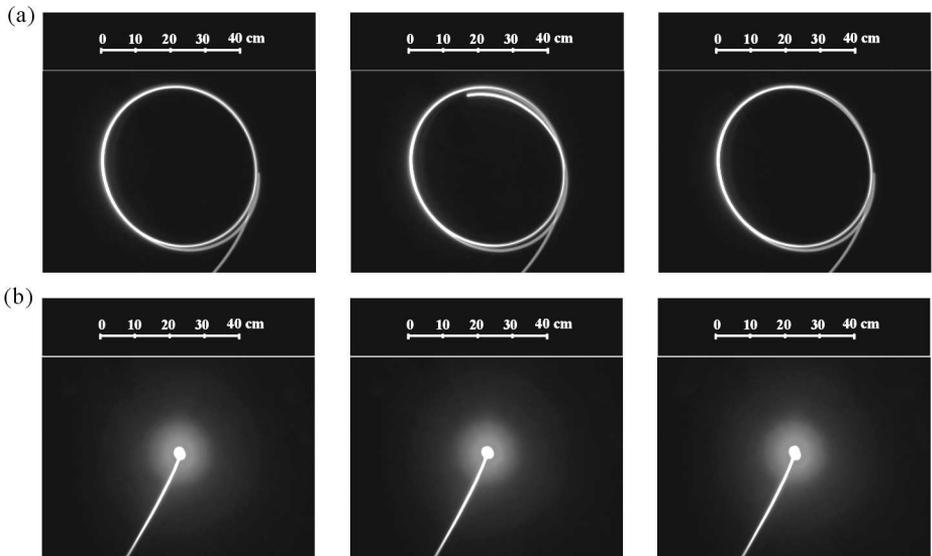
Fig. 8. Experimentally recorded final part of load trajectory for slew of 70° and drive function calculated according to (3.5): (a) – case 1a, (b) – case 1b
