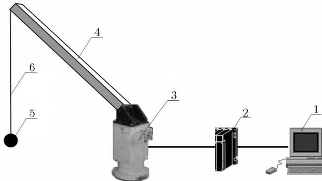
Fig. 4. Schematic diagram of the test stand; 1 – PC with "Test Point" software and DA card, 2 – controller, 3 – manipulator pedestal with servo-motor, gear and rate generator, 4 – jib, 5 – load, 6 – rope
