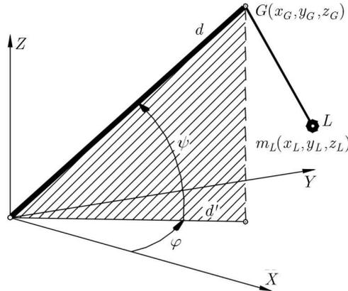
Fig. 1. Simplified model of a crane used for the optimisation task
