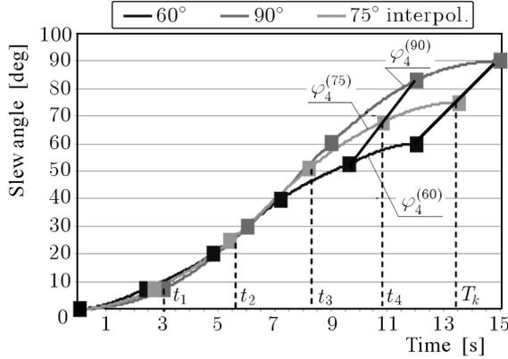
Fig. 3. Example of definition of the drive function for an intermediate slew angle
