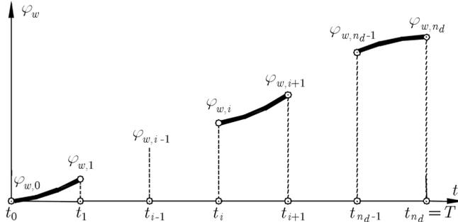
Fig. 2. Function  $\varphi_w(t)$  approximated by spline functions
