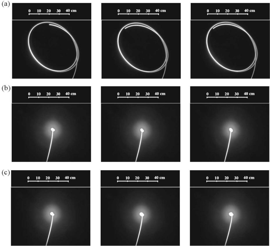
Fig. 10. Experimentally recorded final part of load trajectory for slew of  $80^\circ$  and drive function calculated according to (3.5): (a) – case 3a, (b) – case 3b, (c) – case 3c
