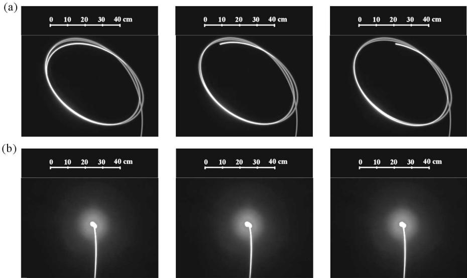
Fig. 9. Experimentally recorded final part of load trajectory for slew of  $90^\circ$  and drive function calculated according to (3.5): (a) – case 2a, (b) – case 2b
