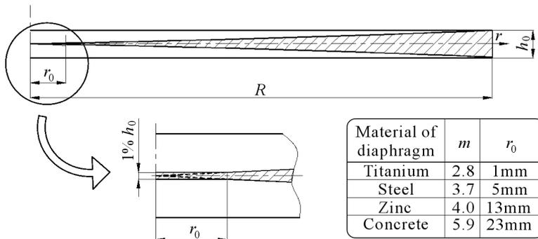
Fig. 2. Lengthwise section along the radial coordinate  $r$  of the plate characterised by geometrical dimensions  $r_0$ ,  $R$ ,  $h_0$
