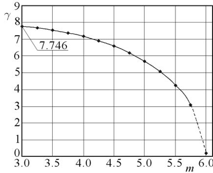
Fig. 1. The curve showing the influence of the plate thickness index on the simplest estimator of the basic frequency coefficient
