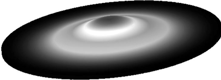
Fig. 3. The base mode of natural vibrations of a titanium diaphragm (330.19 Hz, scale of deformation: 0.025)
