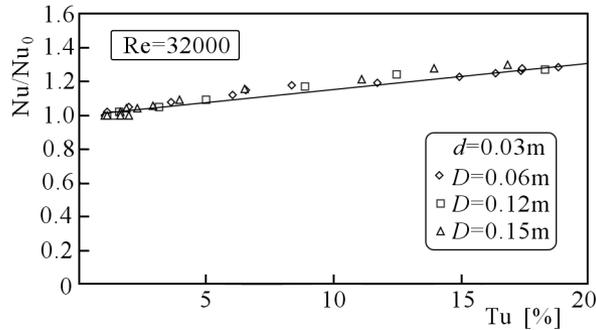
Fig. 3. Distribution of the average heat transfer coefficient on the sphere surface diameter of 0.03 m for different inflow turbulence levels
