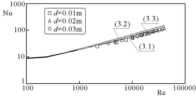
Fig. 2. Distribution of experimental data of the heat transfer coefficient on spheres in comparison with literature data
