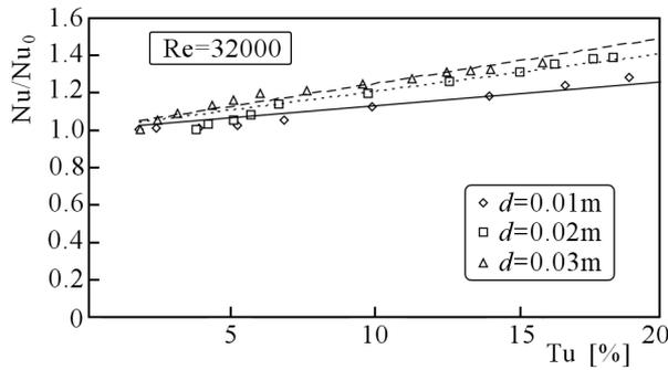
Fig. 6. Trend lines of increasing average heat transfer coefficient on spheres with the surface diameter of 0.01 m, 0.02 m and 0.03 m for different inflow turbulence levels
