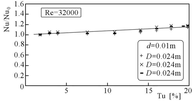
Fig. 5. Distribution of the average heat transfer coefficient on the sphere surface diameter of 0.01 m for different inflow turbulence level
