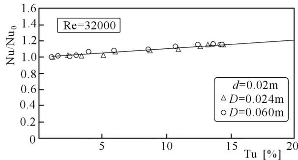
Fig. 4. Distribution of the average heat transfer coefficient on the sphere surface diameter of 0.02 m for different inflow turbulence level
