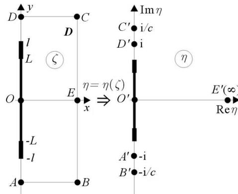
Fig. 2. Scheme of the conformal mapping
