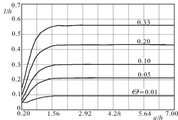
Fig. 4. Regions of geometric parameters in which the solution to the double-periodic problem gives an approximation of the solution corresponding to the periodical rectangle with the relative error not exceeding  $\Theta$
