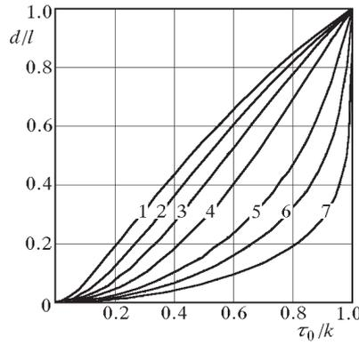
Fig. 3. Length of plastic strips versus load; 1, 2, 3 -  $l/h = 0.9, 0.7, 0.2$ ;
