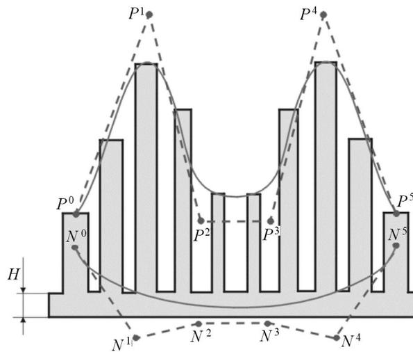
Fig. 10. The method of modelling the shape of the radiator
