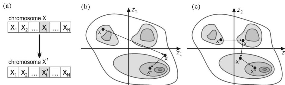
Fig. 5. (a) The scheme of the mutation, (b) searching the uniform mutation, (c) searching the Gaussian mutation
