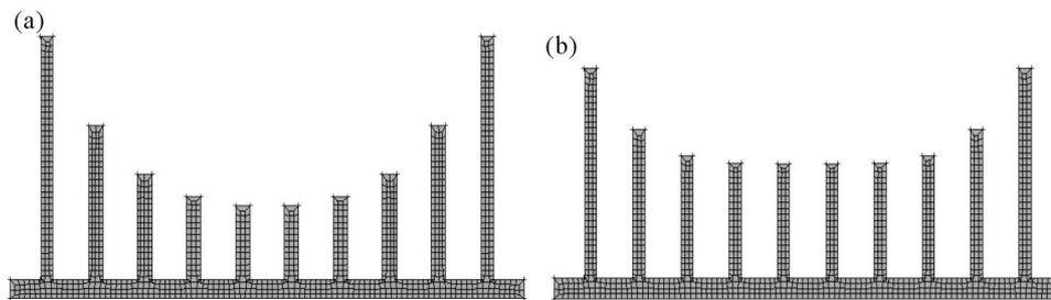
Fig. 12. The optimal shape of the radiator (convection and radiation) for heat flux:
