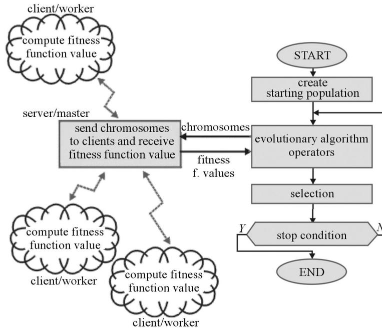
Fig. 7. A flowchart of the parallel evolutionary algorithm
