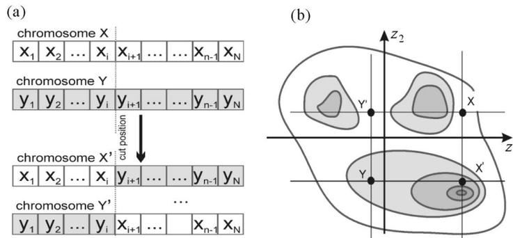
Fig. 6. (a) The scheme of the simple crossover, (b) simple crossover (method of working)
