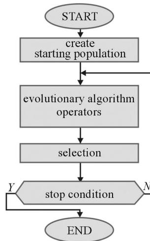
Fig. 4. A flowchart of the sequential evolutionary algorithm
