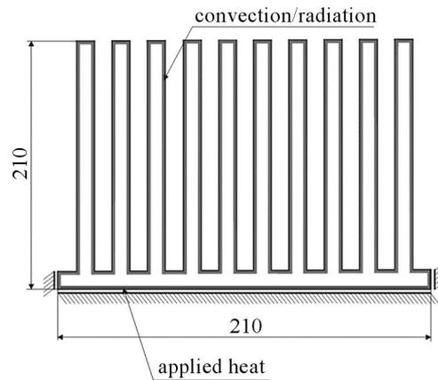
Fig. 9. Geometry and boundary conditions of the analysed heat radiator
