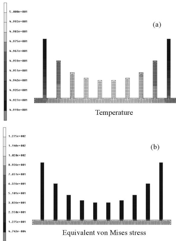
Fig. 13. (a) Temperature distribution in the radiator, (b) equivalent von Mises stress distribution in the radiator (convection and radiation, heat flux  $q = 500 \text{ W/m}^2$ )
