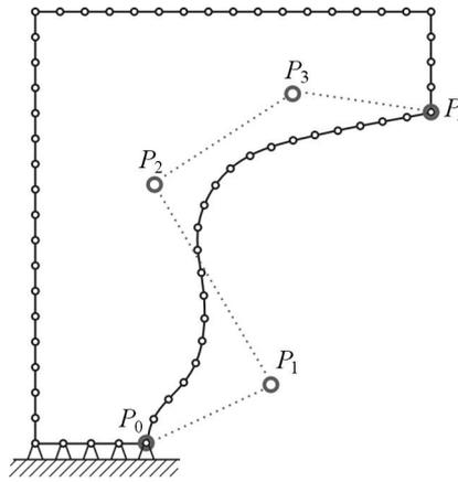
Fig. 3. The modelling of the shape of a boundary by 4th-degree Bezier curves
