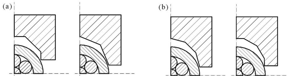
Fig. 10. (a) Octagonal jaw; (b) octagonal-twisted jaw
