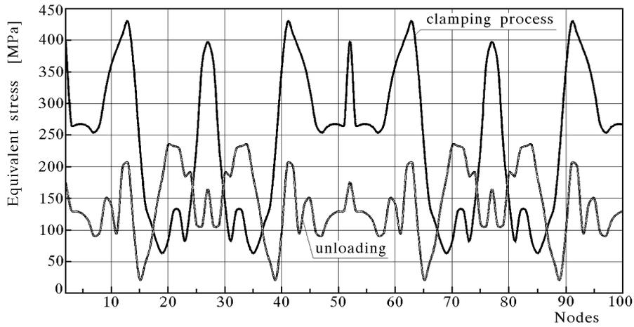
Fig. 14. Reduced residual stress in the dodecagonal clamped joint
