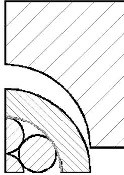
Fig. 13. Nodal displacements in the rope-sleeve contact zone during clamping (black) and unloading (grey)
