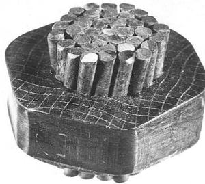
Fig. 1. Rope clamped "into a hexagon"
