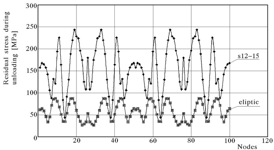
Fig. 15. Reduced residual stress in the dodecagonal and elliptic clamped joint during unloading
