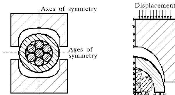
Fig. 9. (a) Symmetry axes of the model; (b) symmetry introduced into the model and boundary conditions
