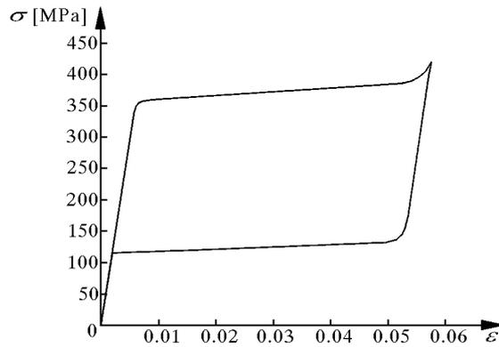
Fig. 6. Nitinol characteristics – 7% deformations
