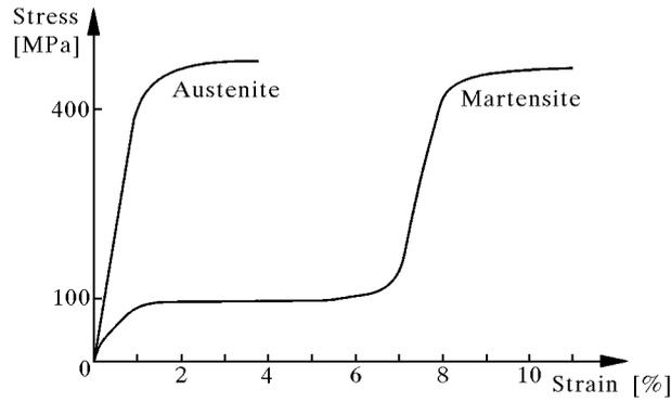
Fig. 5. Nitinol characteristics with phase transitions taken into consideration
