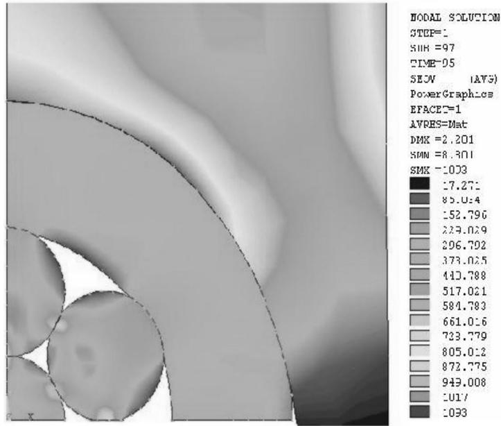
Fig. 11. Residual stresses – the process of clamping
