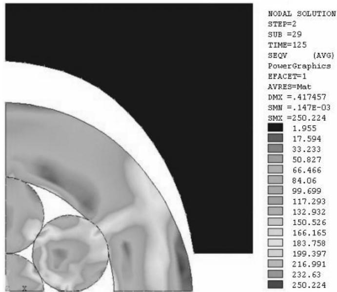
Fig. 12. Residual stresses – the process of unloading
