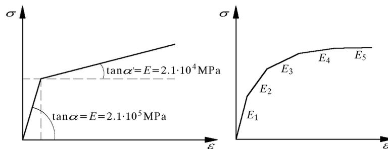
Fig. 3. Bilinear and multi-linear models of the considered material
