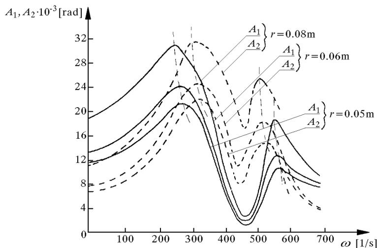
Fig. 9. Resonant curves for various values of the internal radius  $r$  of the discs
