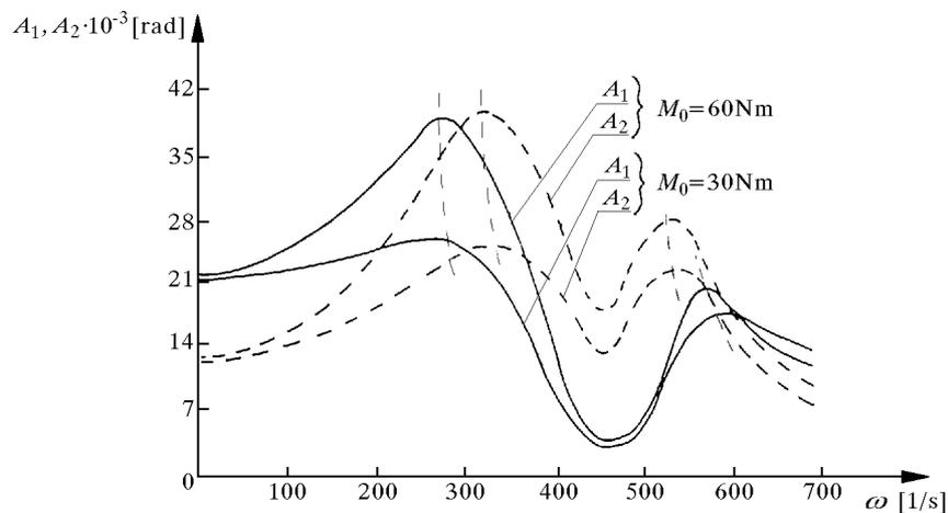
Fig. 6. Resonant curves for various amplitudes of the excitation torque  $M_0$
