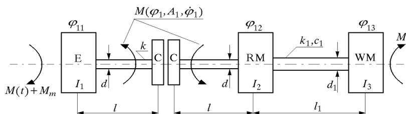
Fig. 1. Physical model of the considered power transmission system
