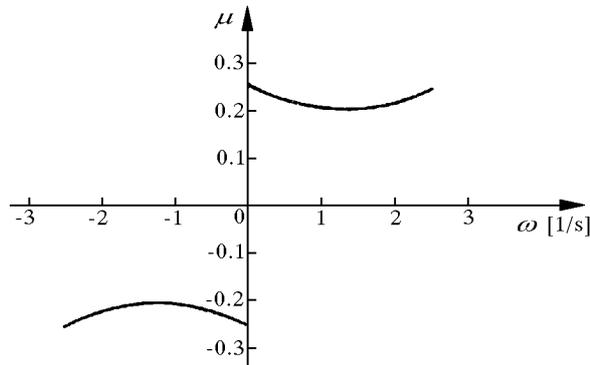
Fig. 5. Variation of the friction coefficient in function of relative speed of sliding discs
