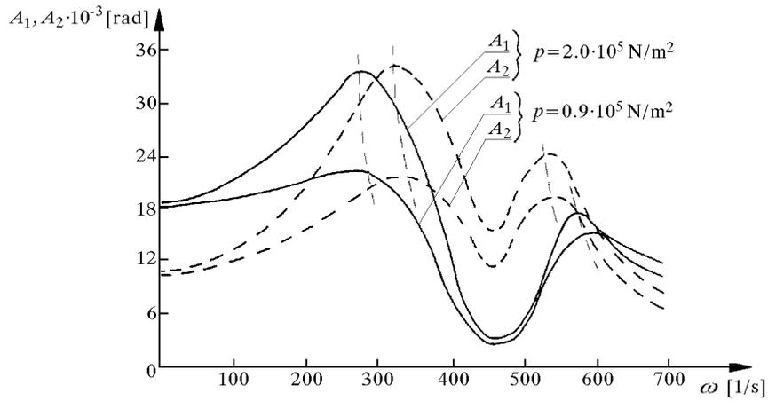
Fig. 7. Resonant curves for various values of the unit pressure  $p$
