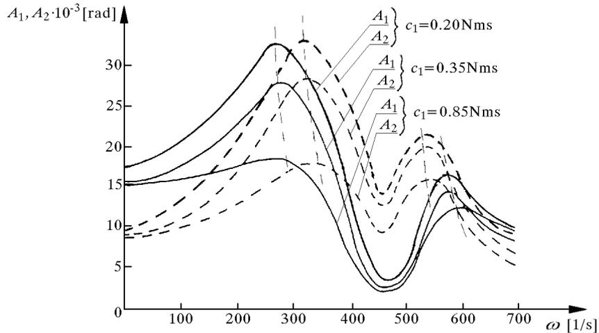
Fig. 8. Resonant curves for various values of the viscotic damping coefficient  $c_1$
