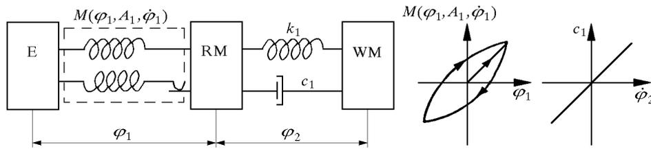
Fig. 2. Mechanical system with a non-linear hysteresis loop and linear viscotic damping reduced to two-degrees-of-freedom
