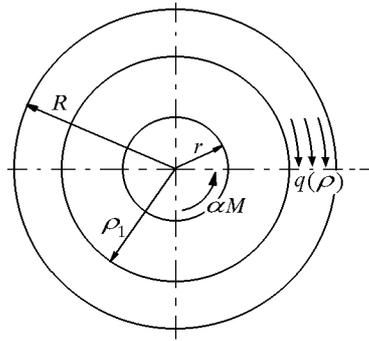
Fig. 3. Load distribution in the frictional pair
