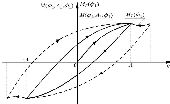
Fig. 4. Hysteresis loops:  $M_T(\dot{\varphi})$ ,  $M(\varphi_1, A_1, \dot{\varphi}_1)$  – moments of friction for kinetic and static friction
