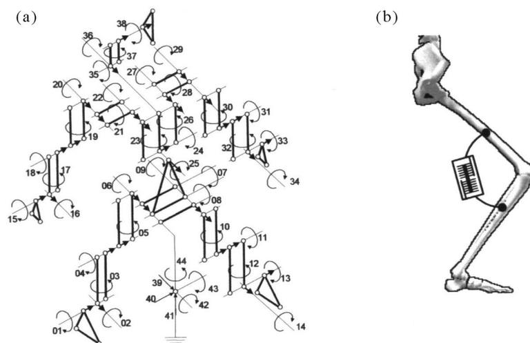
Fig. 3. (a) Degrees of freedom of the biomechanical model; (b) the joint actuator driving the knee joint in the sagittal plane
