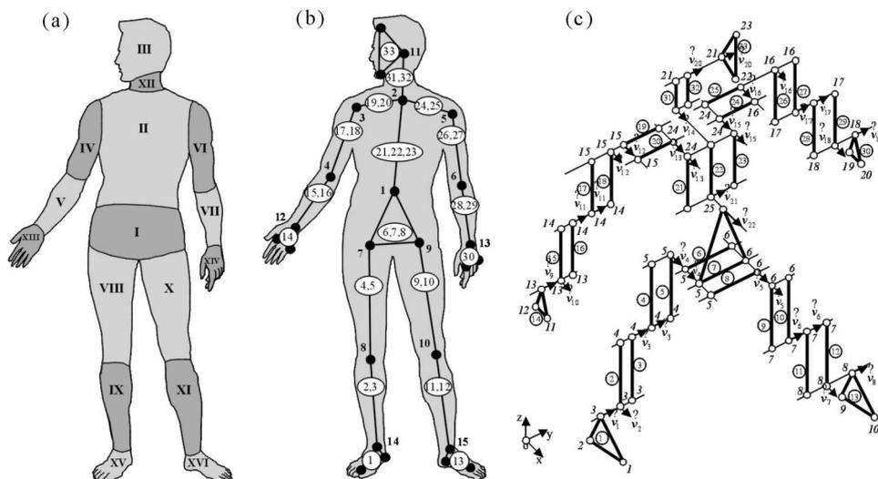
Fig. 1. Biomechanical model. (a) Representation of sixteen anatomical segments; (b) the structure of thirty three rigid bodies (with body numbers inside circles) used to represent the sixteen anatomical segments, and fifteen kinematic joints (with the joint numbers in bold); (c) an exploded view of the kinematic structure of the biomechanical model with indication of the points (represented in italic) and unit vectors
