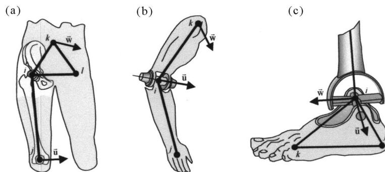
Fig. 2. The model of anatomical joints with natural coordinates: (a) the spherical joint for the hip; (b) the revolute joint for the elbow; (c) the universal joint for the ankle
