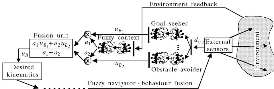
Fig. 10. Basic structure of the fuzzy navigator
