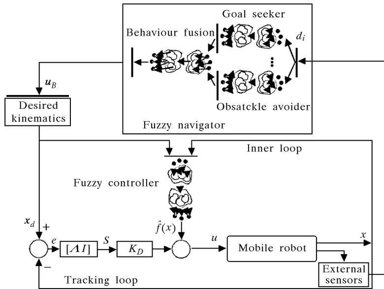
Fig. 9. Architecture of the navigator and controller
