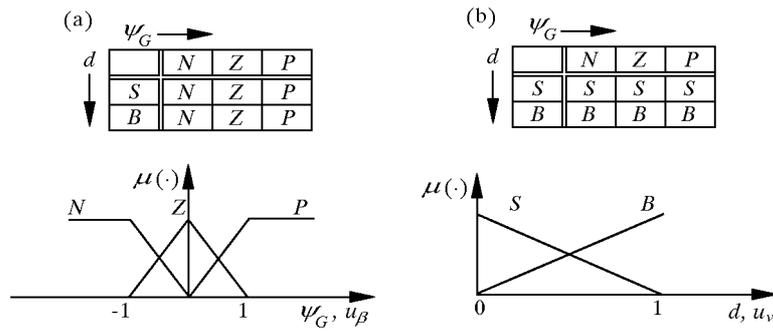
Fig. 5. Angular (a) and linear (b) velocity coefficient rules
