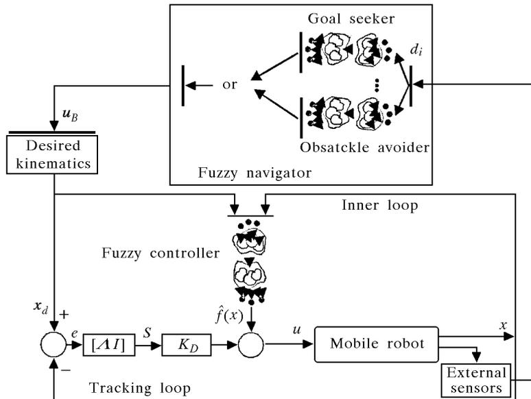
Fig. 2. Navigator and controller
