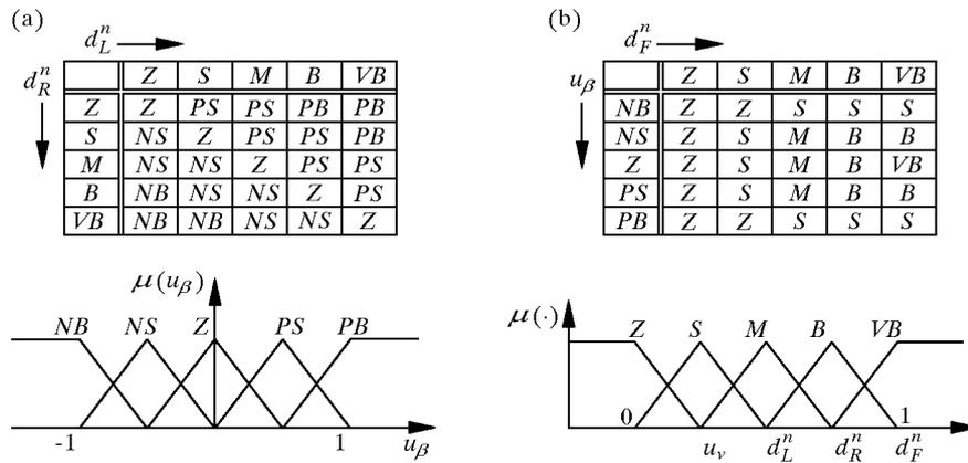
Fig. 3. Angular (a) and linear (b) velocity coefficient rules, respectively
