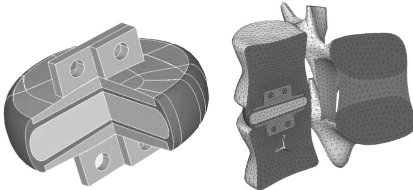
Fig. 13. The artificial disc with the inlay being thick walled container filled with the gel
