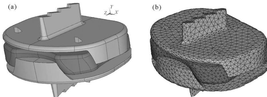
Fig. 15. FE model of the considered new prosthesis: geometrical model (a) and its discretisation (b)
