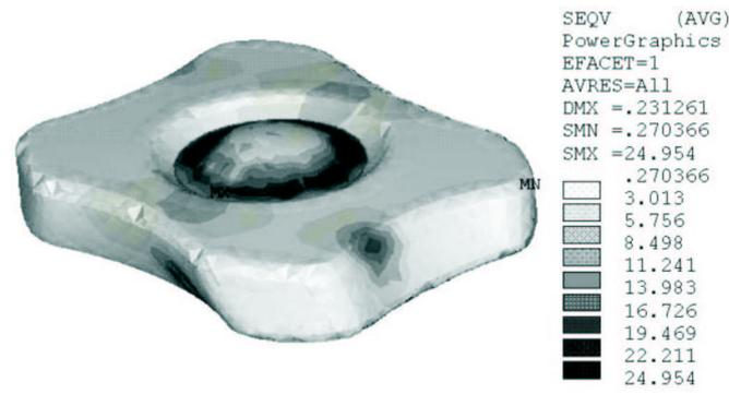
Fig. 16. Von Mises equivalent stresses [MPa] in the polyethylene part of the new prosthesis (compression)
