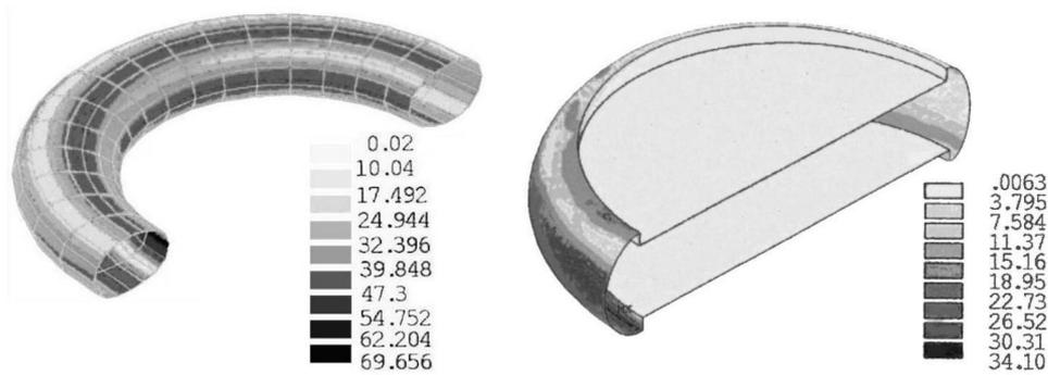
Fig. 14. Von Mises equivalent stresses [MPa] in the polyethylene elements of the new designs (the results correspond to compression analysed for the models shown in Fig. 12 and Fig. 13)
