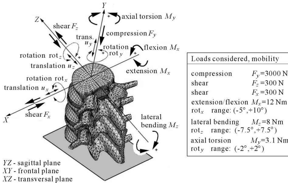
Fig. 3. Some of the parameters defining mechanical requirements for the total disc prosthesis
