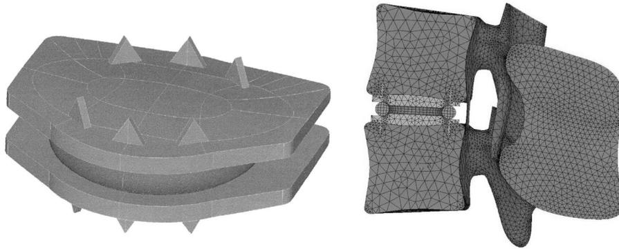
Fig. 12. The artificial disc with toroidal middle
