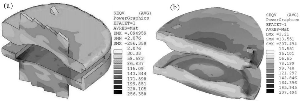
Fig. 7. Von Mises equivalent stresses [MPa] in metal plates of prostheses: (a) ProDisc, (b) Charite III
