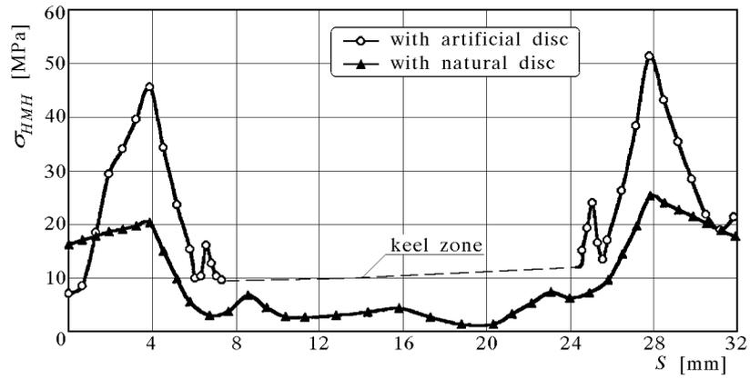
Fig. 10. Von Mises equivalent stress distribution [MPa] on the top surface of the lower vertebra along the path at the symmetry plane  $YZ$  (see Fig. 9)
