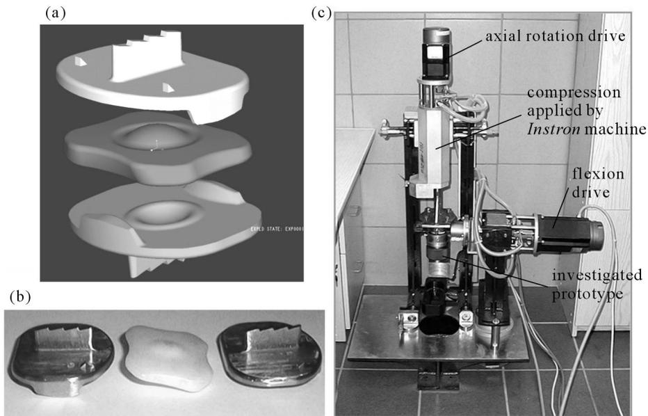
Fig. 17. The CAD model of the new design (a), the prototype (b) and the experimental stand (c)
