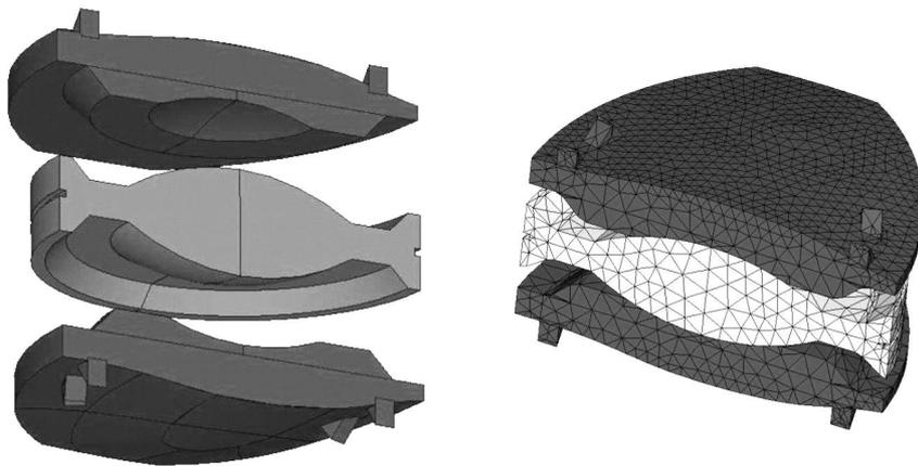
Fig. 6. FE model of the Charite III artificial disc
