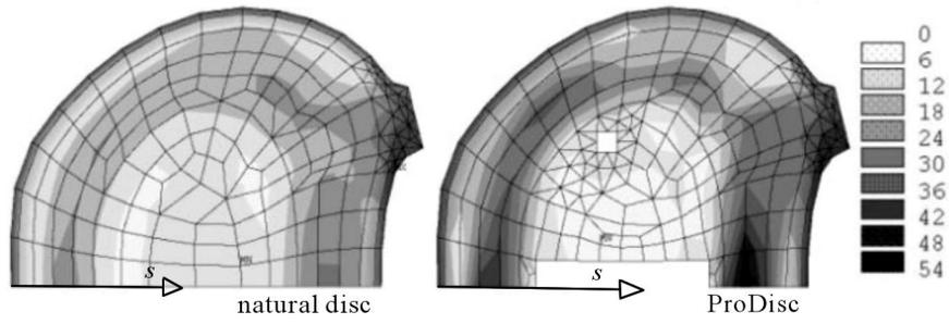
Fig. 9. Von Mises equivalent stress distribution [MPa] on the top surface of the lower vertebra for the compression 3000 N
