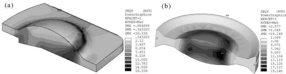
Fig. 8. Von Mises equivalent stresses [MPa] in the polyethylene inlays of prostheses: (a) ProDisc, (b) Charite III
