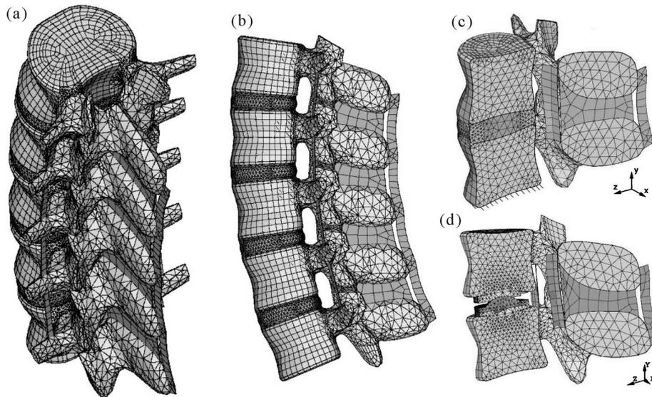
Fig. 4. Finite element model of a spine segment: (a) FE mesh, general view, (b) cross-section in the sagittal plane, (c) cross-section of the motion segment with a natural disc, (d) cross-section of the motion segment with an artificial disc
