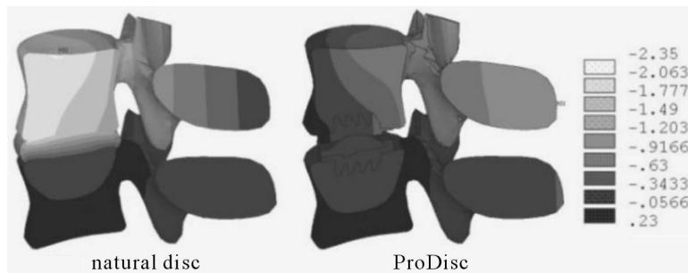
Fig. 11. Vertical displacement [mm] distribution due to the 3000 N compression
