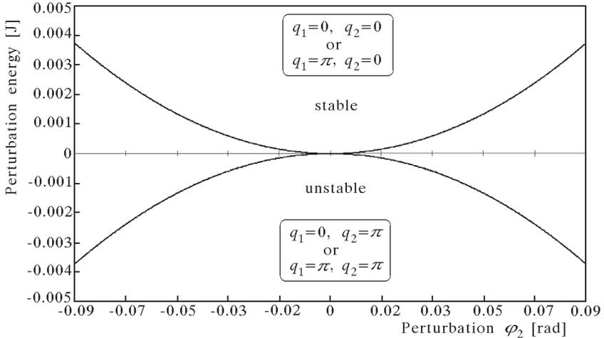
Fig. 2. Perturbation potential energy distribution in the case of an unstable and stable point
