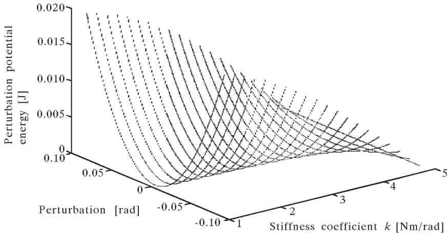
Fig. 13. Finding the stability boundary of the system
