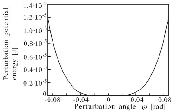
Fig. 11. Perturbation of the system for the coefficient  $k$  corresponding to the stability boundary
