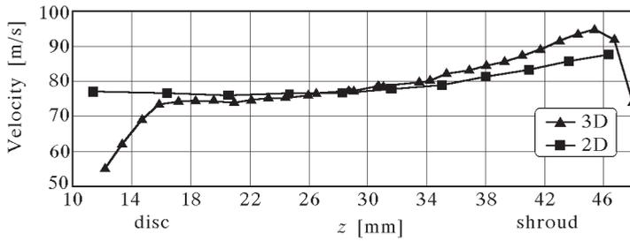
Fig. 10. Velocity distribution at the inlet section
