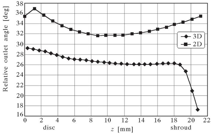
Fig. 12. Velocity angle at the impeller outlet
