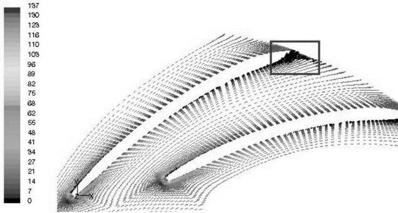
Fig. 17. Velocity vectors close to the shroud
