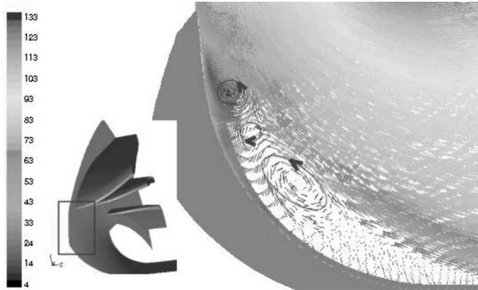
Fig. 3. Separation zone upstream to the leading edge
