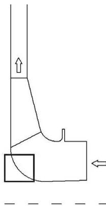
Fig. 2. Radial compressor (meridional section)
