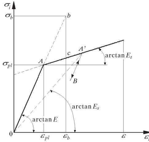
Fig. 2. Bilinear stress-strain relation
