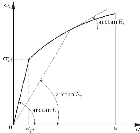
Fig. 3. Nonlinear stress-strain relation
