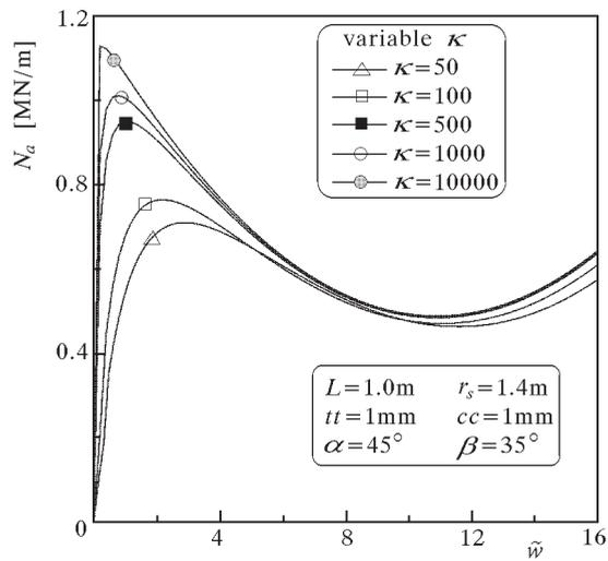
Fig. 7. Longitudinal force  $N_a$  versus deflection  $\tilde{w}$
