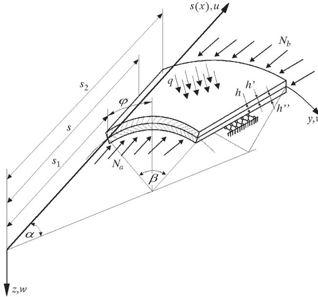
Fig. 1. Subject of consideration – bilayered open conical shell
