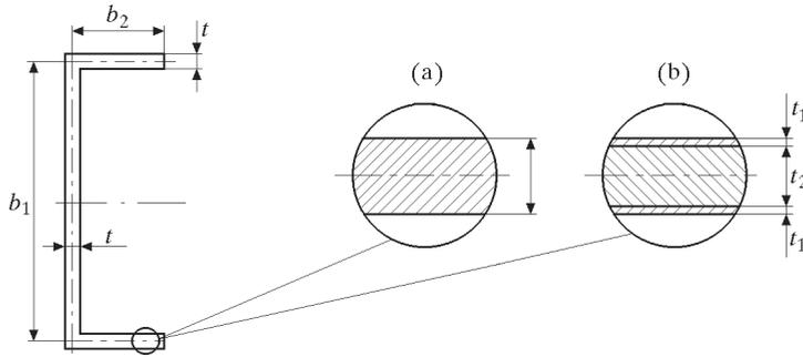
Fig. 1. Two cases of manufactured channels: composite material (a); steel+composite+steel (b)
