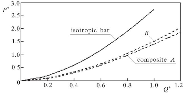
Fig. 7. Nondimensional load parameter  $P^*$  versus  $Q^*$  for the isotropic and composite materials
