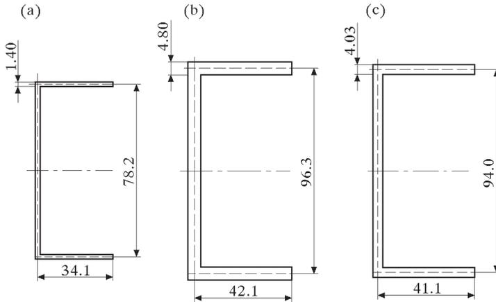
Fig. 4. Optimal profiles of channels with the same weight ( $Q^* = 0.2$ ) for  $L = 1$  m:
