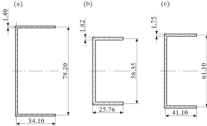
Fig. 3. Optimal profiles of channels with the same area ( $Q^* = 0.2$ ) for  $L = 1$  m:
