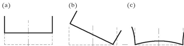
Fig. 2. Considered buckling mode: (a) overall flexural mode; (b) flexural-torsional mode; (c) local mode
