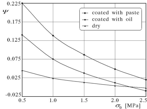
Fig. 5. Characteristics of the energy dissipation coefficient  $\Psi$  of the tested contact joints
