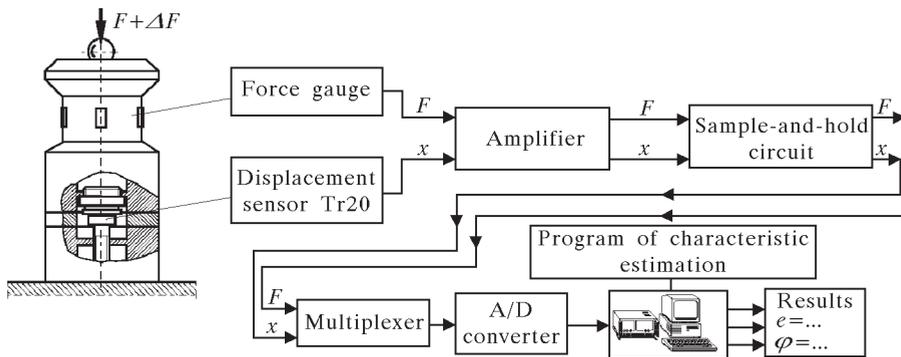
Fig. 1. Block diagram of the system for recording and processing signals
