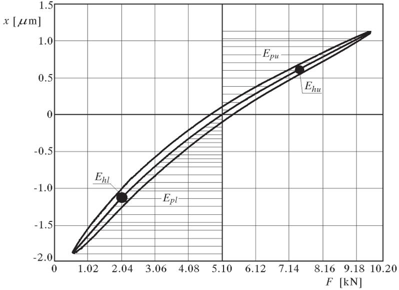
Fig. 4. Graphical interpretation of the integral definition of the energy dissipation coefficient
