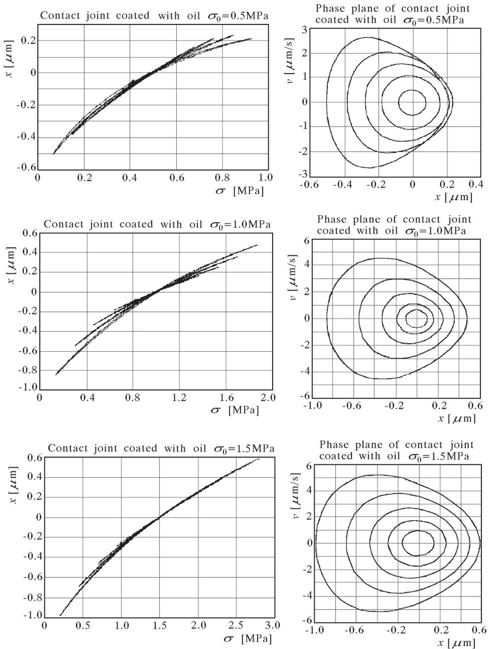
Fig. 3. Deformability characteristics and phase plane of motion in the tested contact joint coated with oil
