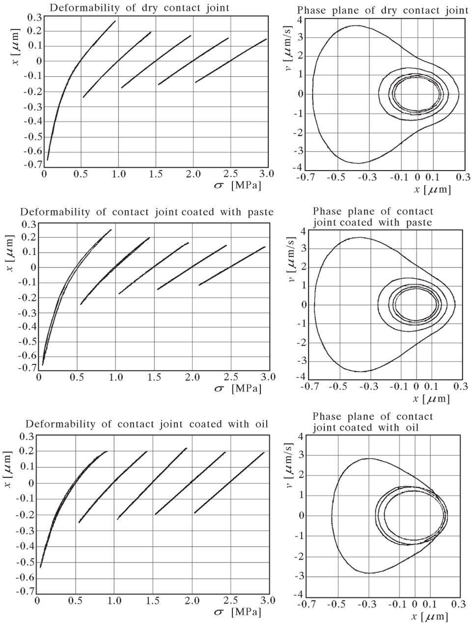
Fig. 2. Deformability characteristics and phase plane of motion in the tested contact joint for  $\sigma_m = 0.425$  MPa and  $0.5 < \sigma_0 < 2.5$  MPa
