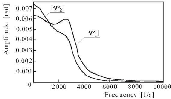
Fig. 6. Amplitude-frequency characteristic of torsional vibration of the sandwich shaft with damping in the interlayer at the point  $x_0 = 0.5l$
