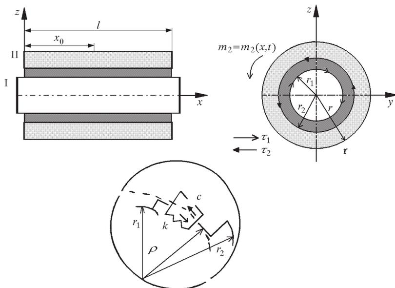
Fig. 1. Model of torsional vibration of the sandwich shaft with damping in the interlayer
