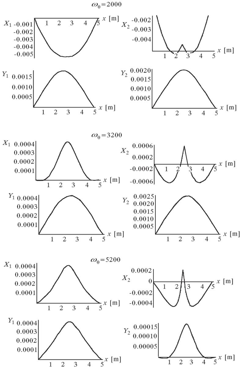
Fig. 5. Complex modes of stationary forced vibrations of shafts I and II
