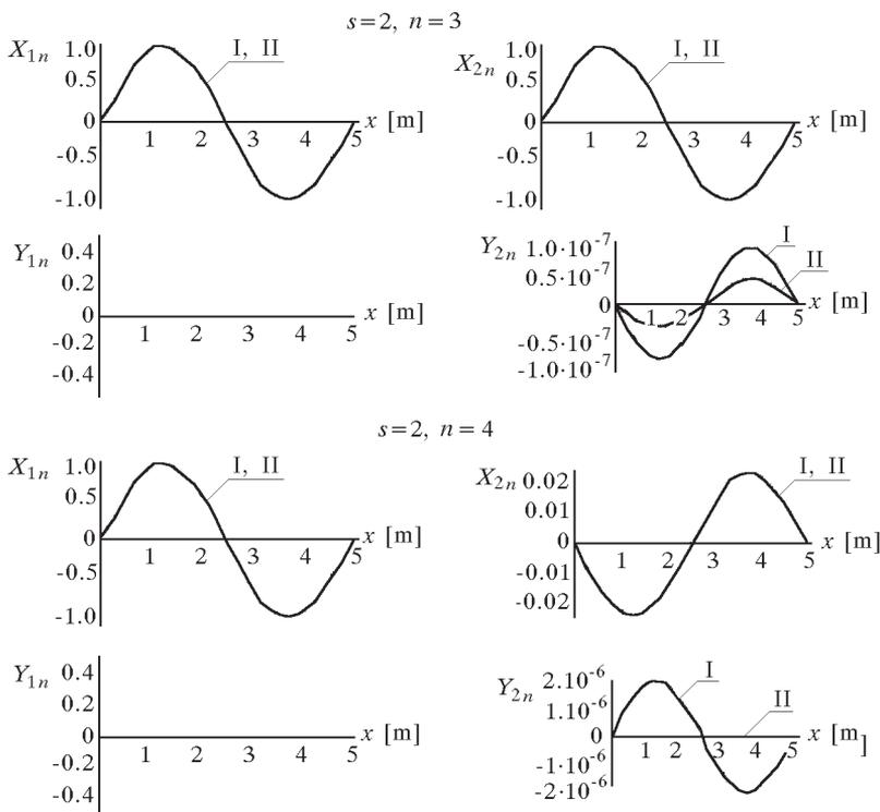
Fig. 4. Complex modes of free vibrations of shafts I and II for  $s = 2, (n = 3, 4)$  – variants I, II
