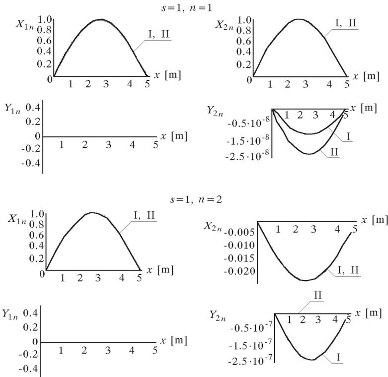
Fig. 3. Complex modes of free vibrations of shafts I and II for  $s = 1, (n = 1, 2)$  – variants I, II
