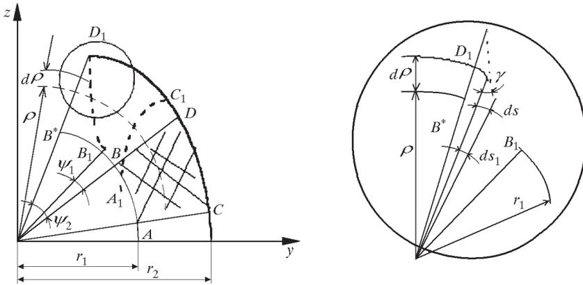
Fig. 2. Deformation of a separated segment of the interlayer
