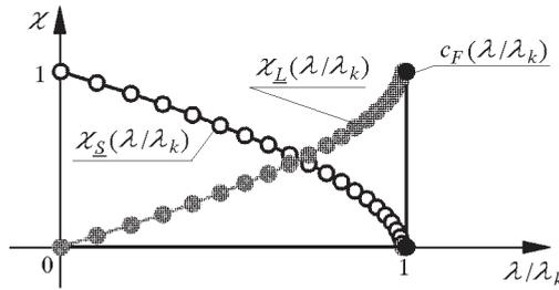
Fig. 5. Areas: desirable  $\underline{S}$ , limit  $\underline{L}$  and undesirable  $F$  in the case of a snap-through type of loss of stability
