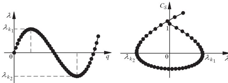
Fig. 4. Equilibrium path and scalar rigidity parameter of the Mises truss
