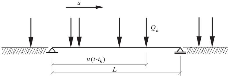
Fig. 1. The beam loaded by a random train of forces travelling in the same direction, all with equal, constant velocities  $u$
