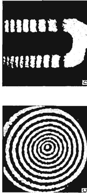
Fig. 9. Demonstration of preprocessing steps (A) smoothed correlogram, (B) image (A) divided by a „very-low” pass filtered, (C) binary image of (B), (D) binary image of the in-plane displacement of a tuning-fork
