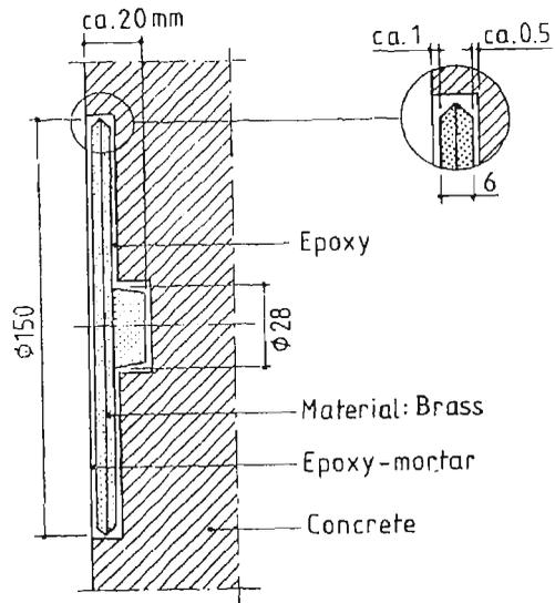
Fig. 2. Installation of normal stress cell in wall
