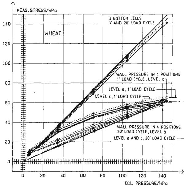
Fig. 8. Stress state in wheat filled calibration chamber
