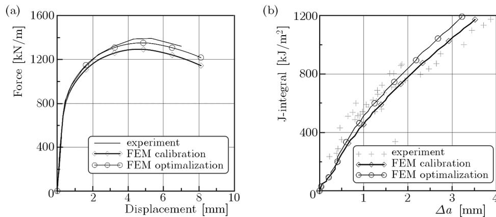
Fig. 9. Results of the three-point bend test and numerical simulation; (a) force-load-point-displacement, (b)  $JR$ -curve
