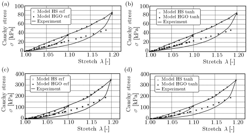
Fig. 2. (a), (b) The Mullins effect – circumferential strip, (c), (d) the Mullins effect – longitudinal strip
